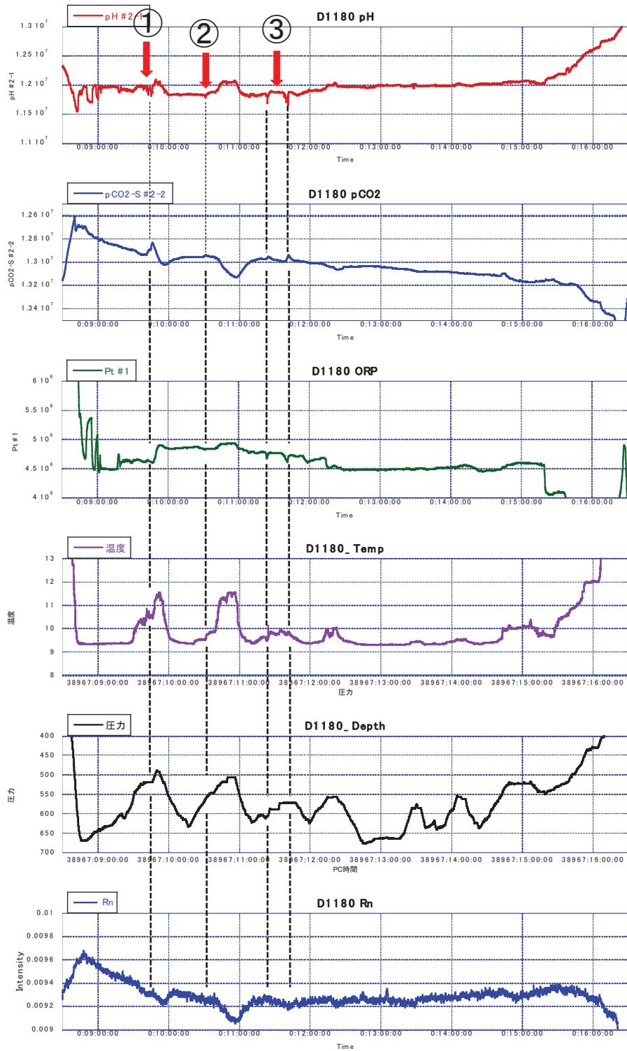
Fig. 15 *In-situ* Time Variation of Multi Chemical Parameter Sensors on Dive 1180
