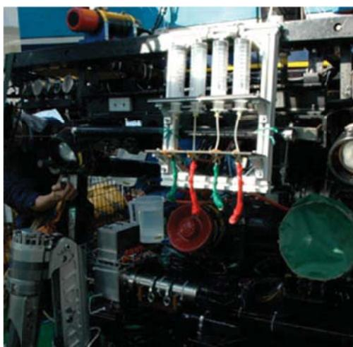
Fig. 10 Syringe Water Samplers
