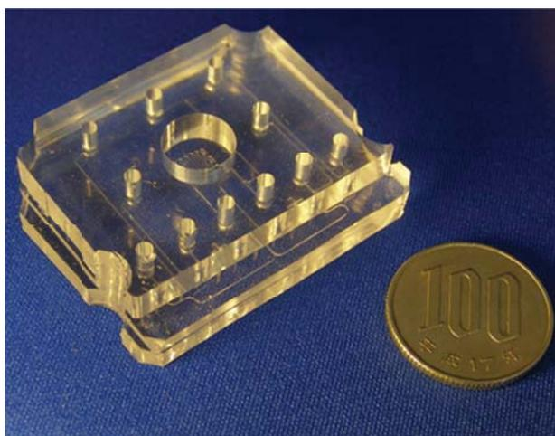
Fig. 5 Microfluidic Device for IISA-Mn
