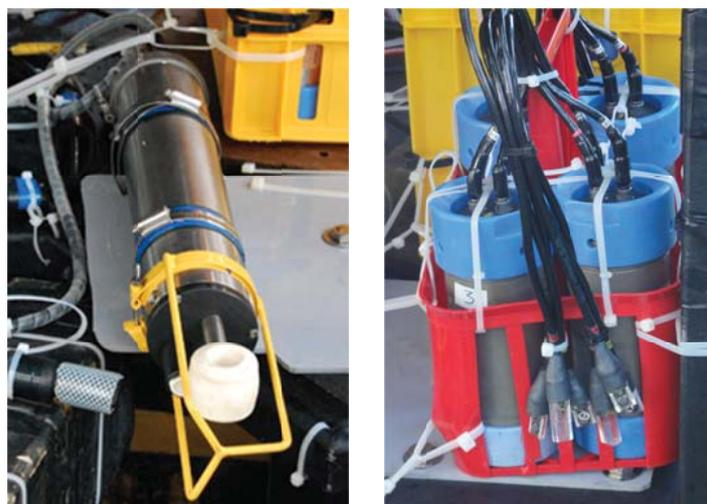
Fig. 8 Multisensor (Left: CTD, Right: pH/pCO<sub>2</sub>/ORP Sensor)
