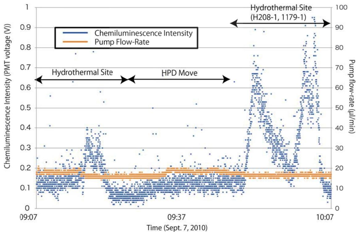
Fig. 11 Chemiluminescence Intensity (Mn Concentration) Anomalies Observed during the Dive #1179. Blue: Chemiluminescence Intensity, Orange: Pump Flow-Rate
