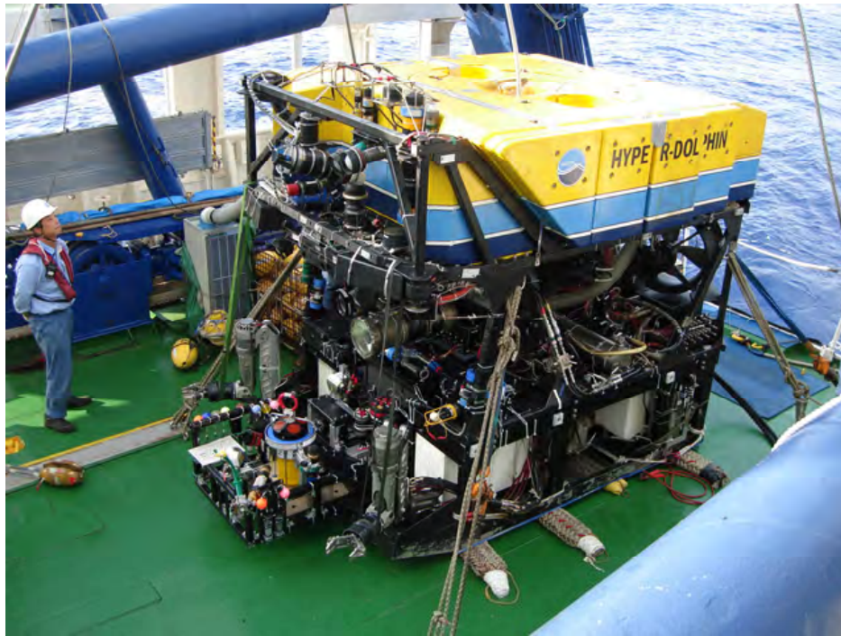
Fig. 25 HPD with payload apparatuses and sensors for dive #1318
