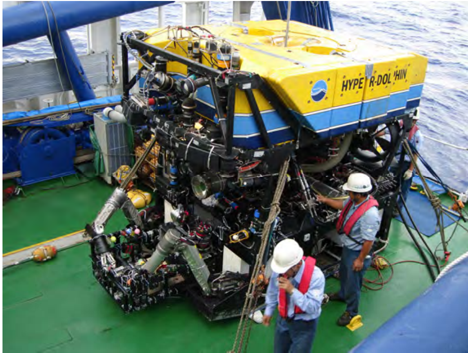
Fig. 31 HPD with payload apparatuses and sensors for dive #1319
