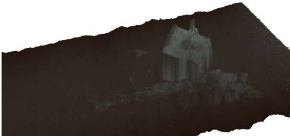
Fig. 8 3D model generated from images recorded at an altitude of 4.5m by the Firefly camera
