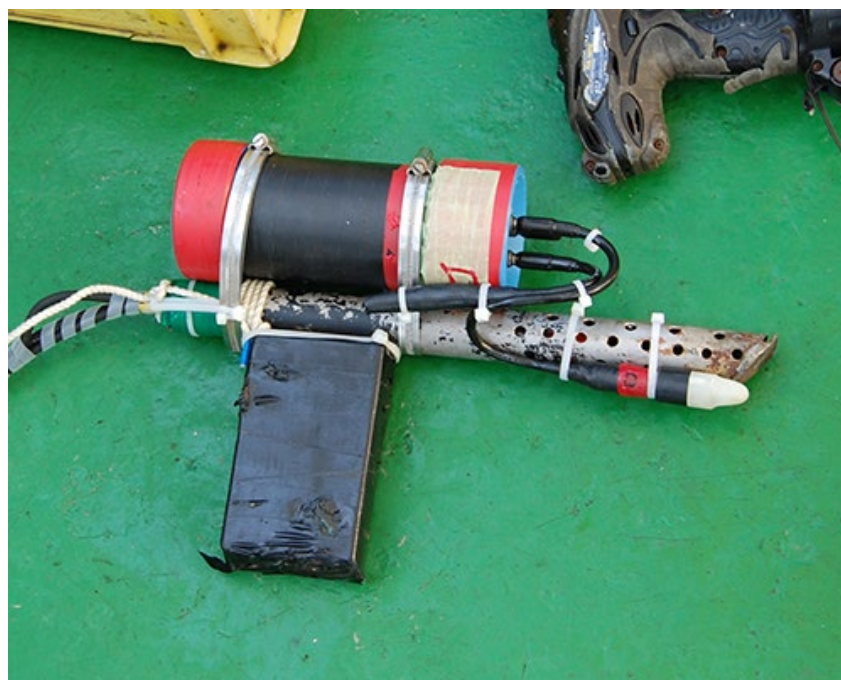
Fig. B ISFET-pH sensor bundled with DEEP-POTE H 2 S sensor head
