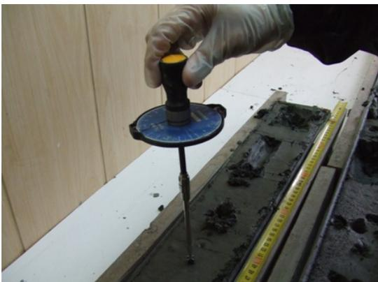
Photo 3.10 Vane shear test
