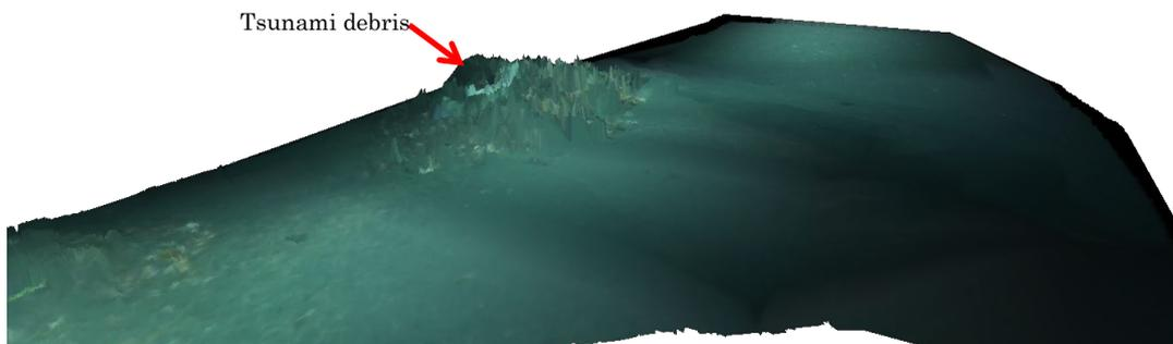
**Fig. 3 3D map of the Surveyed area with Tsunami debris visible.**
