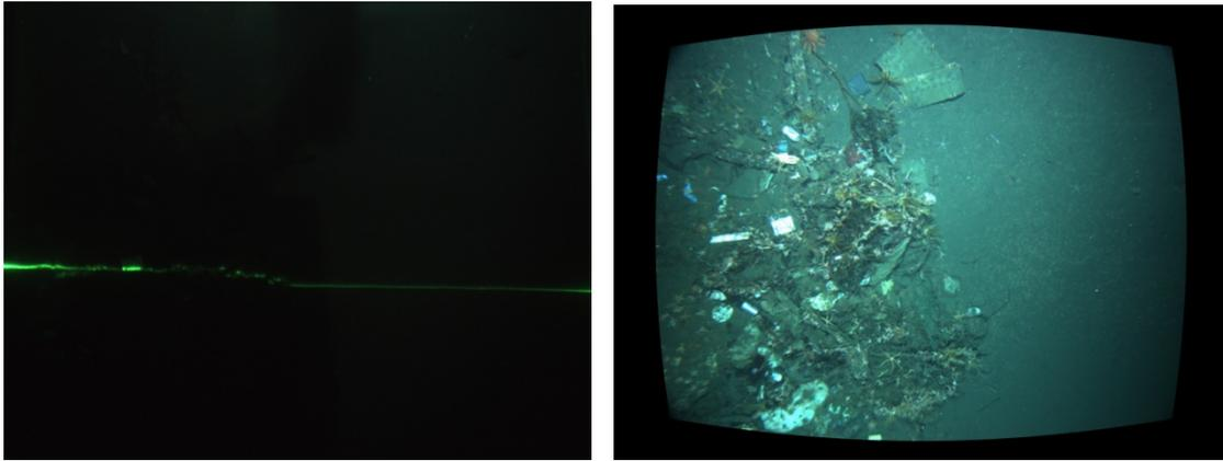
**Fig. 2 Laser Profile and Flashed image used to generate 3D map**
