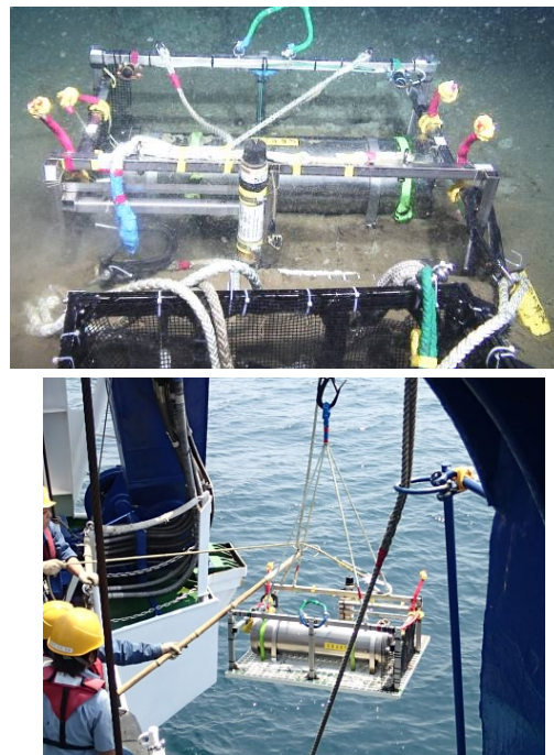
Fig. 5-9. Retrieval operation of the hydrophone array system. Top photo shows in sea water at 2080 m taken by HPD's camera, and lower photo was
