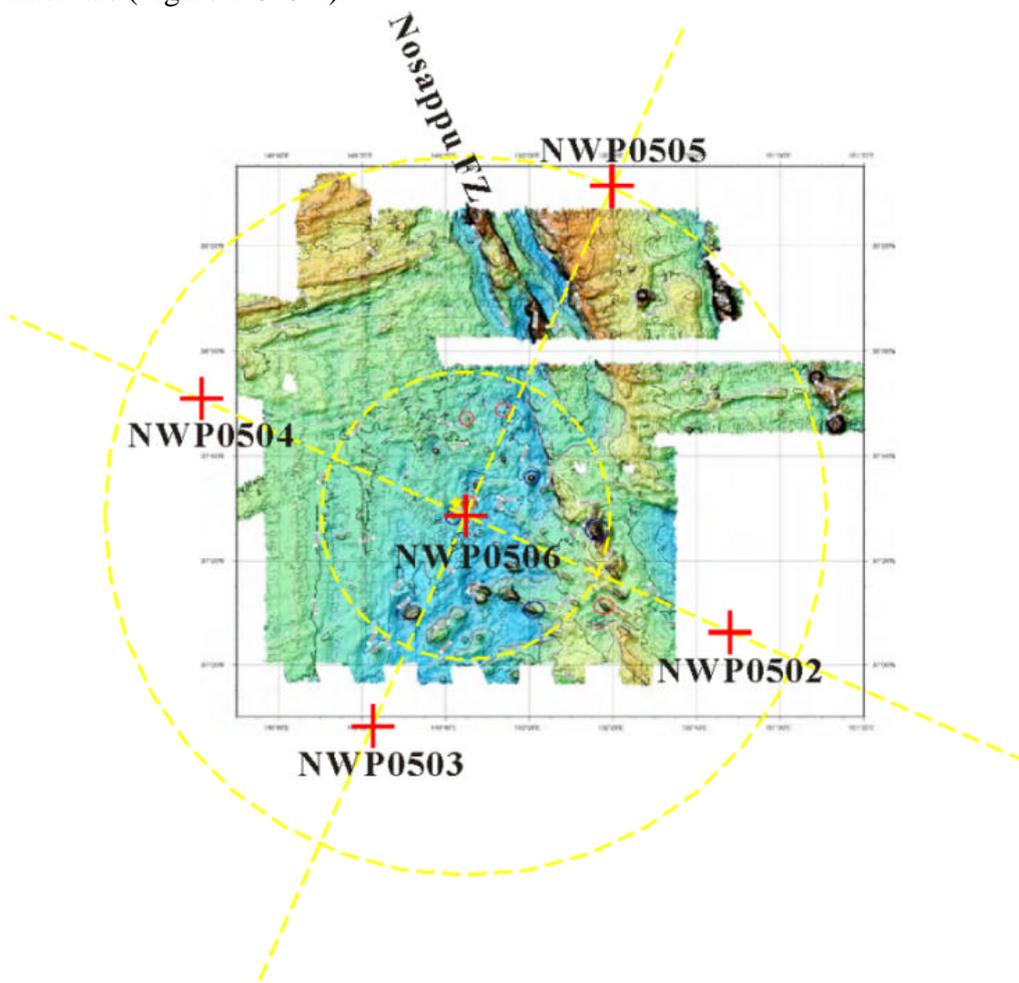
**Figure 1-3-6-1.** Bathymetry map and the MT site locations around the “Petit Spot” area. Red crosses are the locations where OBEMs were deployed in this cruise. Dashed lines are the directions parallel to and perpendicular to the Pacific plated motion and the circles centering on Yukawa knoll with diameters of 100 km and 250 km, respectively.
