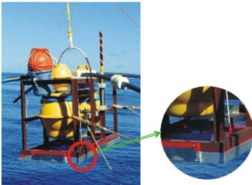
**Figure 4-1-2.** Recovery buoy-rope system. The stopper is fixed between lead weight and OBEM aluminum frame. Once the lead weight is released, the stopper becomes free and the buoy rises forward.
