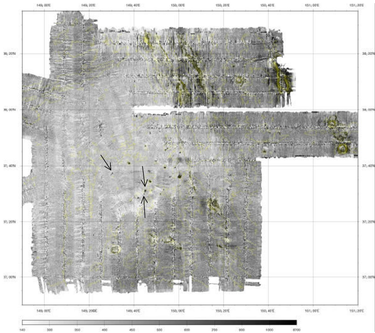
**Figure 5-1-2.** Back-scatter image of the B-area by the KR04-08 cruise. This is the same scale and area as Figure 5-1-1. Three dive points are shown by arrows.
