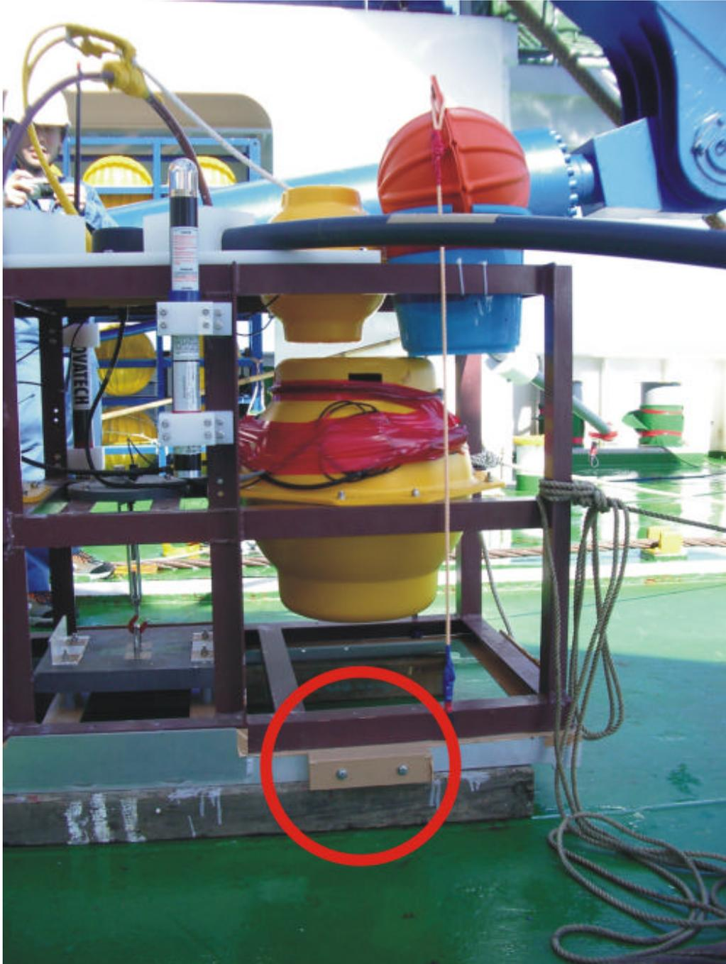
**Plate 5-2-1.** Additional weight settlement. The weight is attached in the side of the glass sphere for the battery and the recovery buoy.
