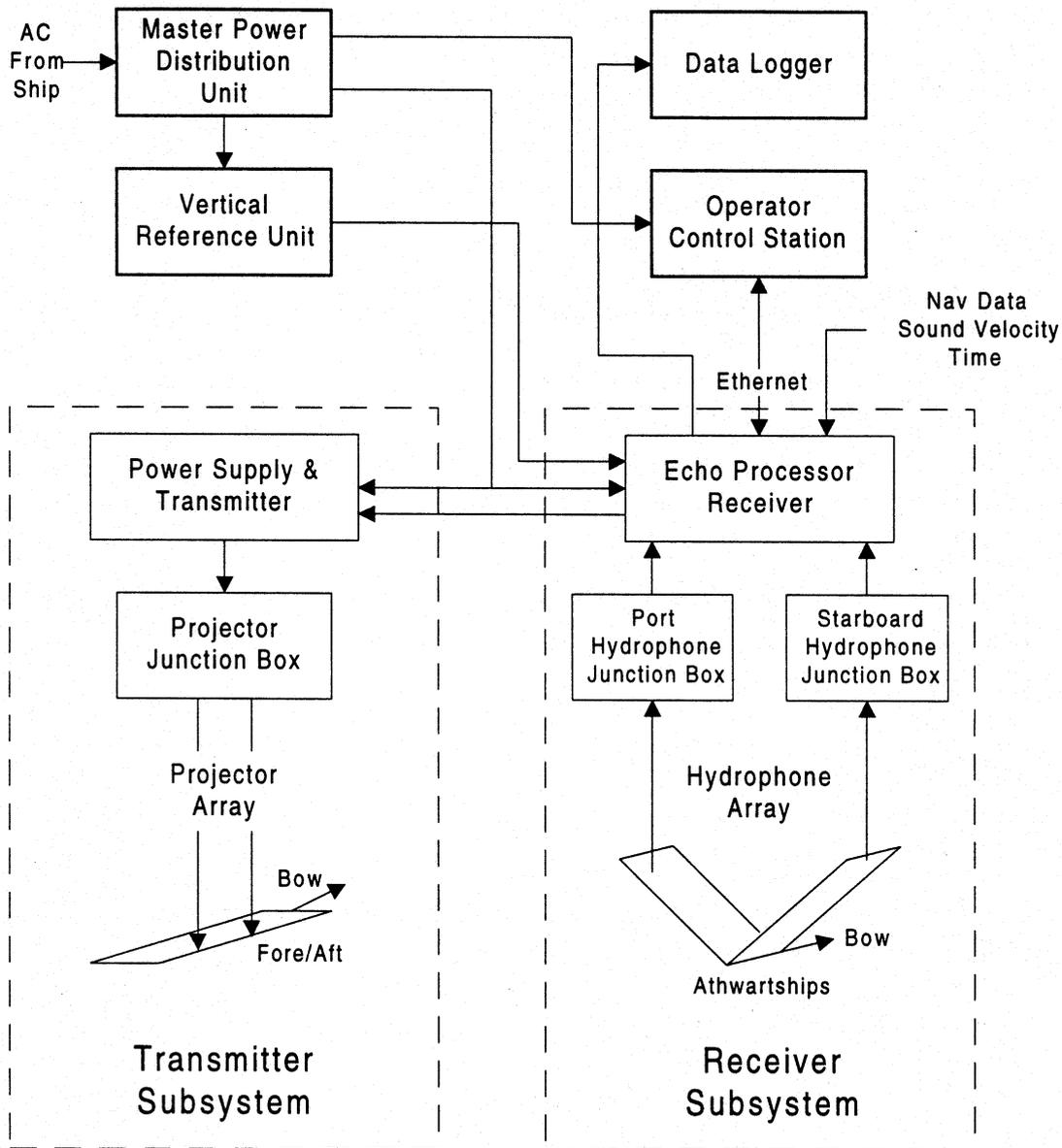
**Figure 4-3-1.** Basic diagram of the SAE BEAM system
