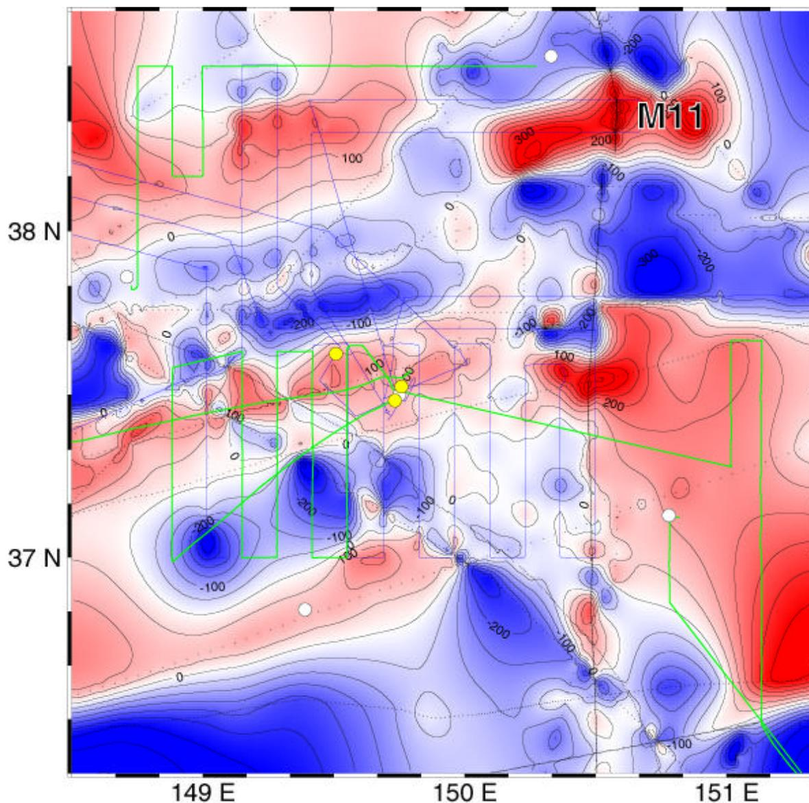
**Figure 5-5-2.** Magnetic anomaly map of the B-area. Contour lines are plotted every 50 nT. Red shade indicates positive anomaly and blue shade indicates negative anomaly. Green lines show ship tracks obtained in the YK05-06 cruise. Blue lines show the KR03-07 and KR04-08 ship tracks. Dotted lines correspond to ship tracks from NGDC data used in this compilation. Yellow circles mark Shinkai dives and white circles mark OBEM stations. White heavy white lines delineate the Nosappu Fracture Zone.
