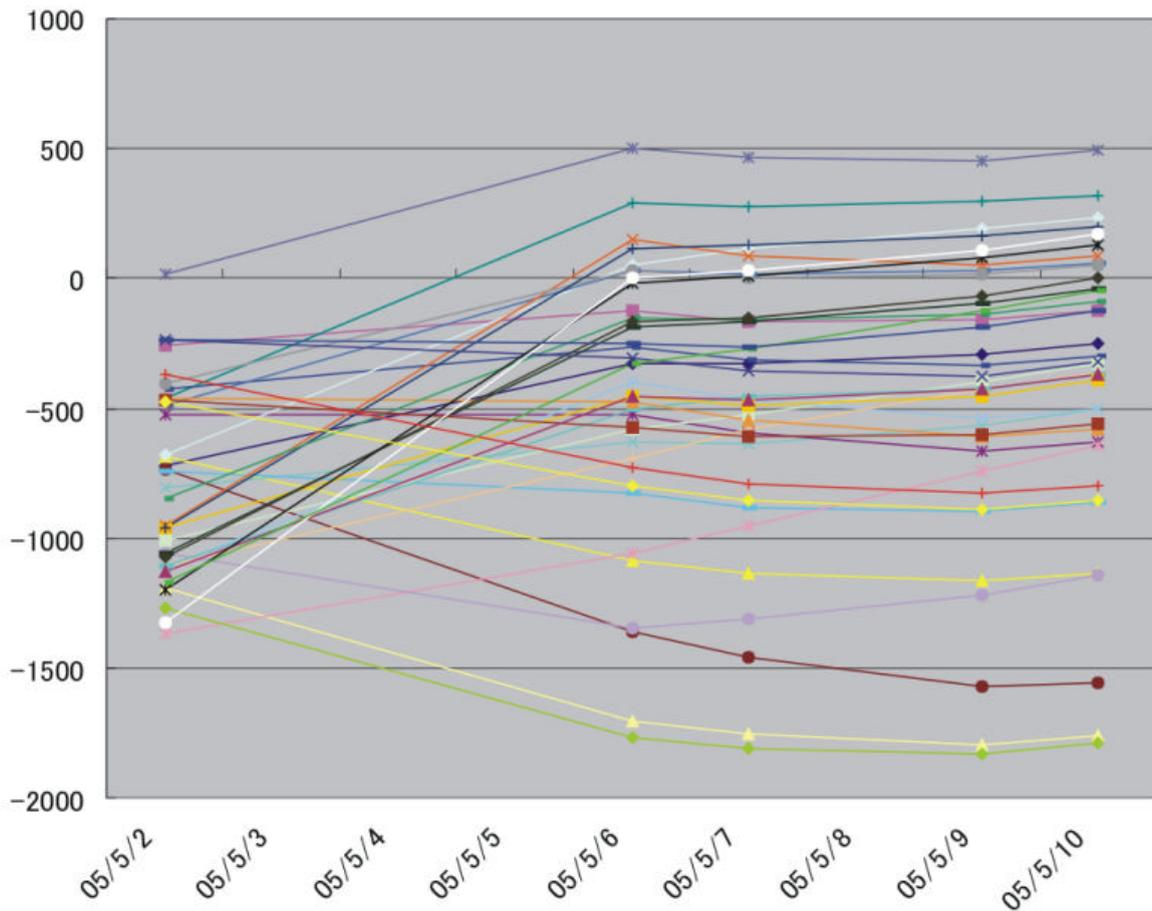
**Figure 5-2-3.** Aging test of the electrodes. Number of all electrodes are 38. The common electrode's ID was 0503044. The unit of vertical axis is micro-volts. The aging test started on 2nd, May, 2005. Each 5 electrodes were selected on the day before the deployment day.
