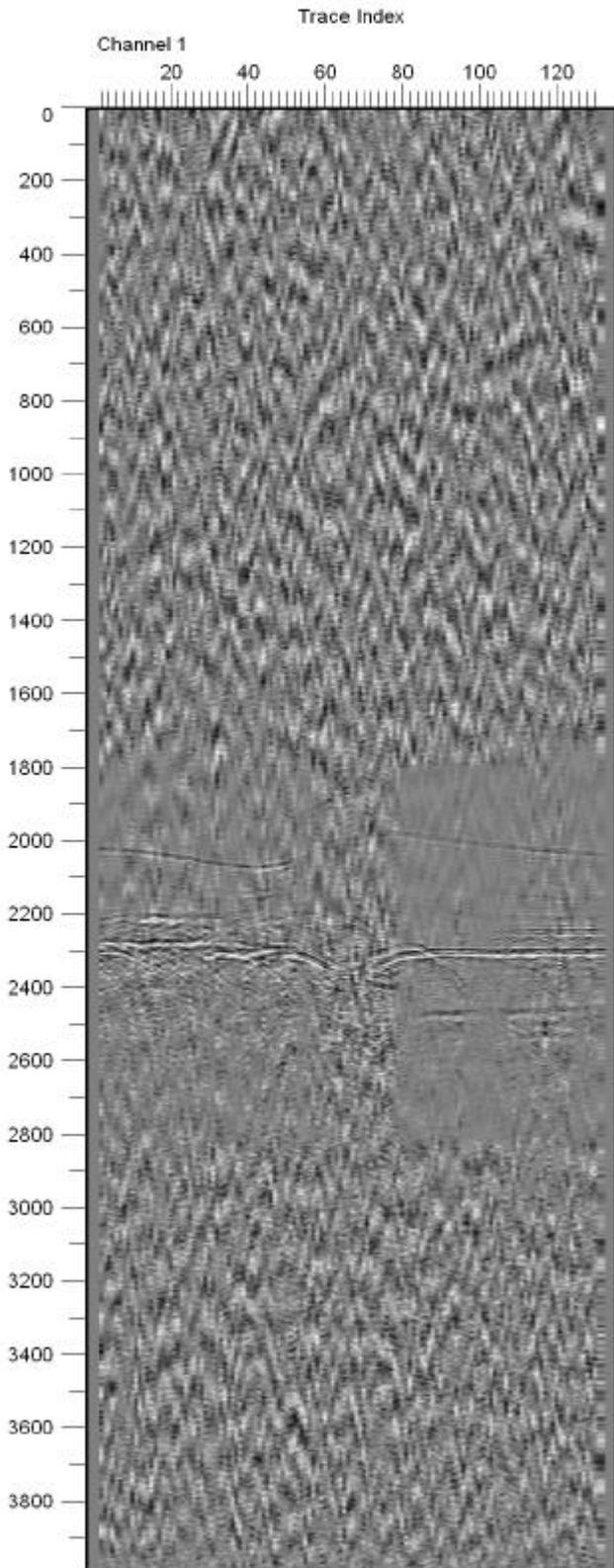
**Figure 5-3-2.** Seismic profile Line A-B. Vertical axis shows two-way travel time (msec). 6000 msec is subtracted from true TWT.
