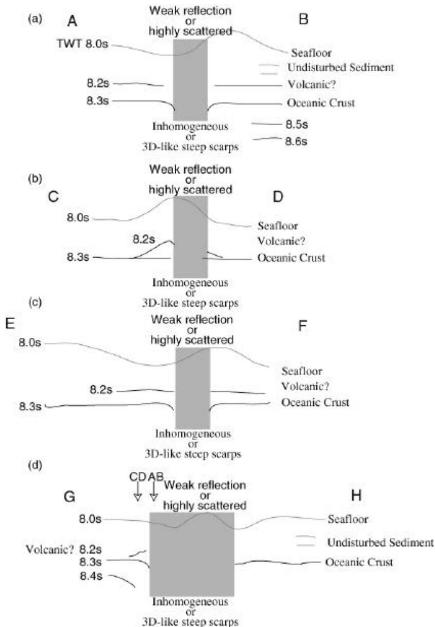
**Figure 5-3-10.** Interpretations of the seismic profiles. (a) Line AB (Yukawa Knoll: NNW to SSE). (b) Line CD (Yukawa Knoll: WSW to ENE). (c) Line E-F (North Yukawa Knoll: NW to SE). (d) Line G-H (North Yukawa Knoll: SW to NE). AB and CD show the cross points at Line A-B and C-D, respectively. Note that shape and scale are inaccurate because of TF's poor ability in illustration.
