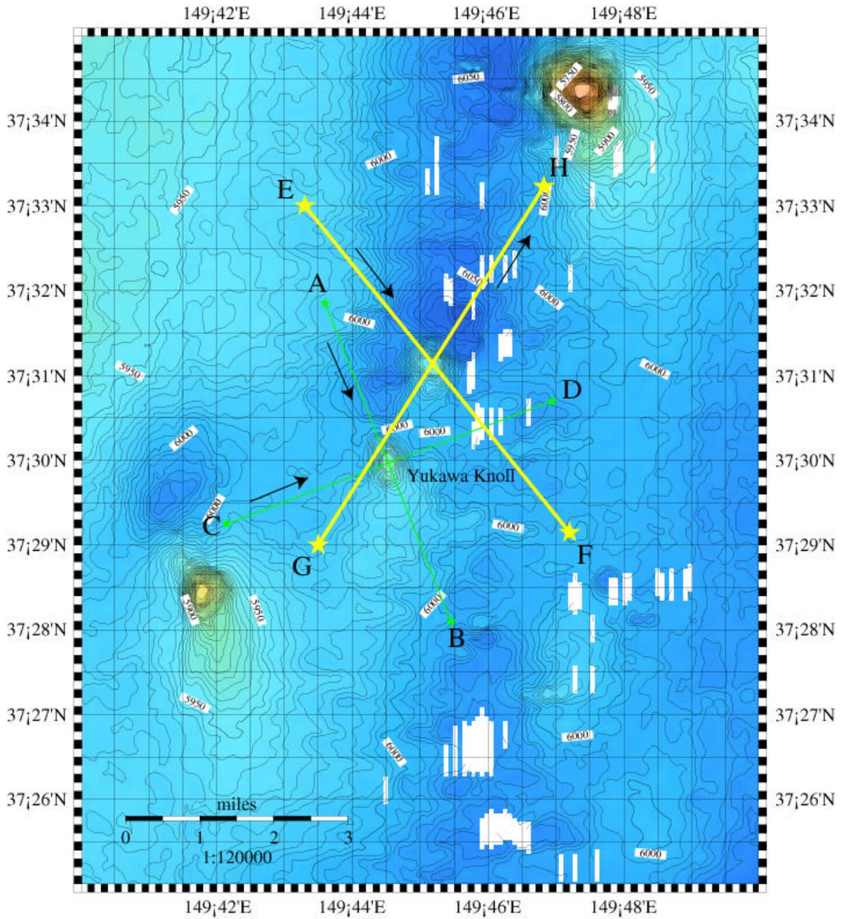
**Figure 5-3-1.** Ship tracks of the single channel seismic reflection survey. Arrows show the ship's direction of movement.
