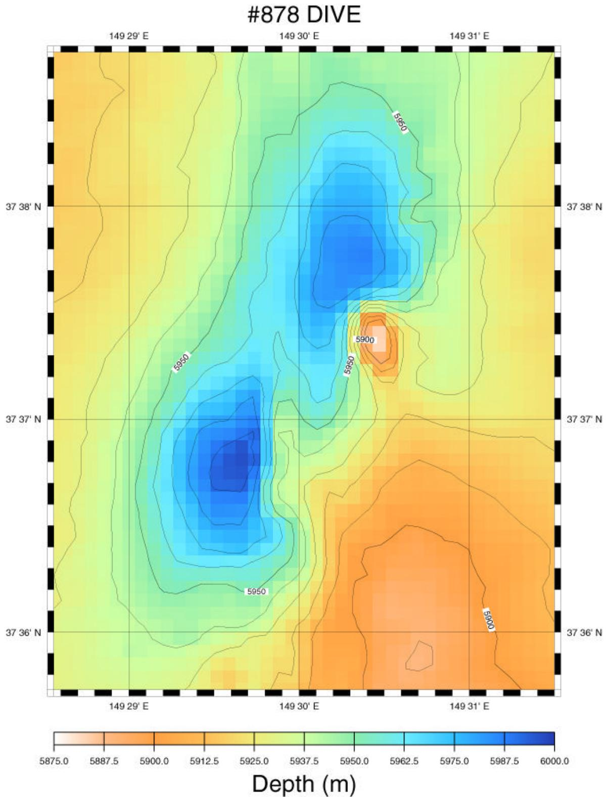
**Figure 5-1-2-1.** Detail bathymetric map around the dive#878 site. Eastern slope in these two craters show high back-scatters. The small knoll was found by the site-survey of this dive.
