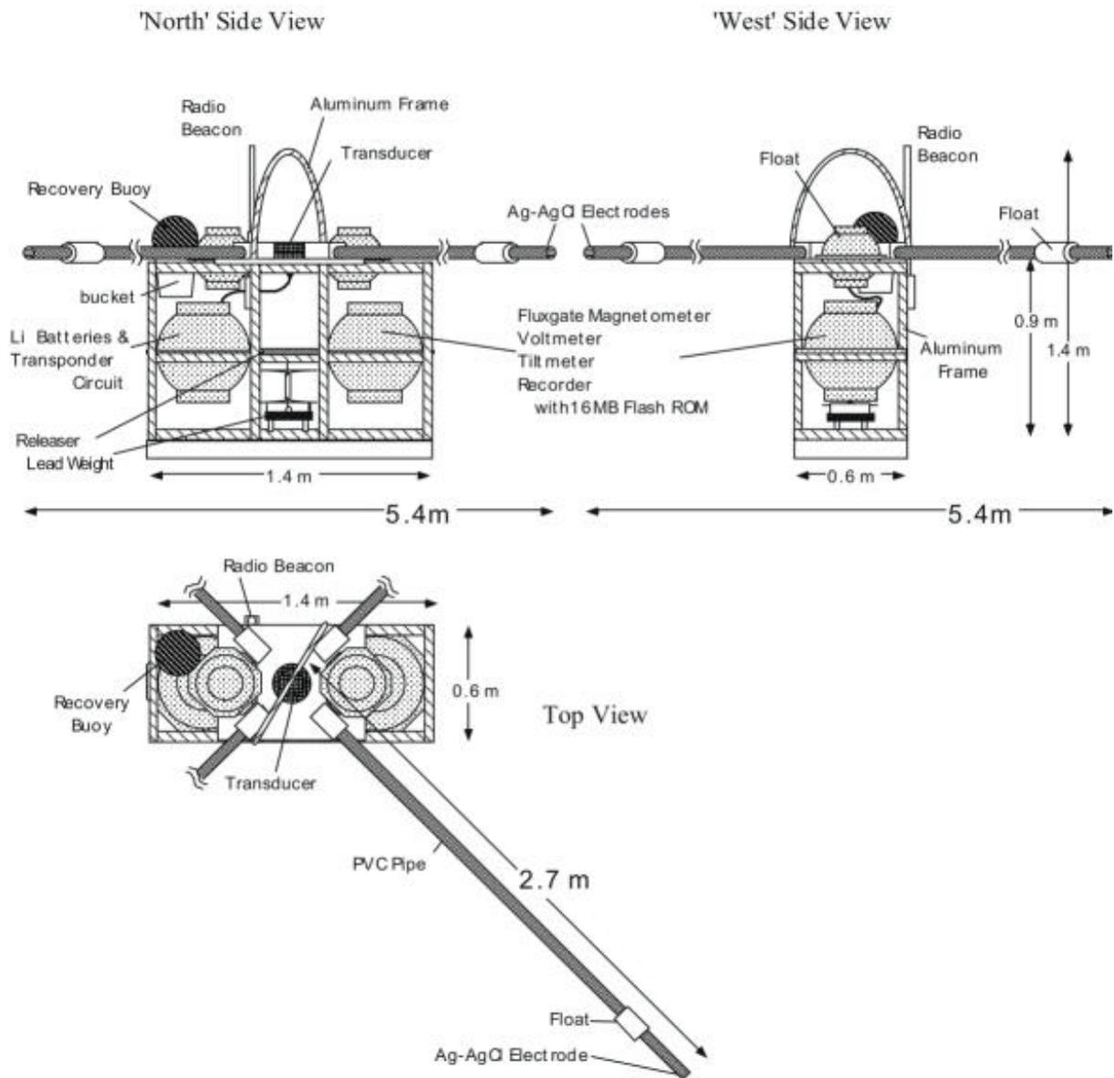
**Figure 4-1-1.** Side and top views of the two-glass-sphere type's OBEM. The 1st generation of this type was manufactured in 1996. Its total weight in air is 130kg (without the lead weight). Main lead weight the mass of which is 40 kg is attached in deployments.
