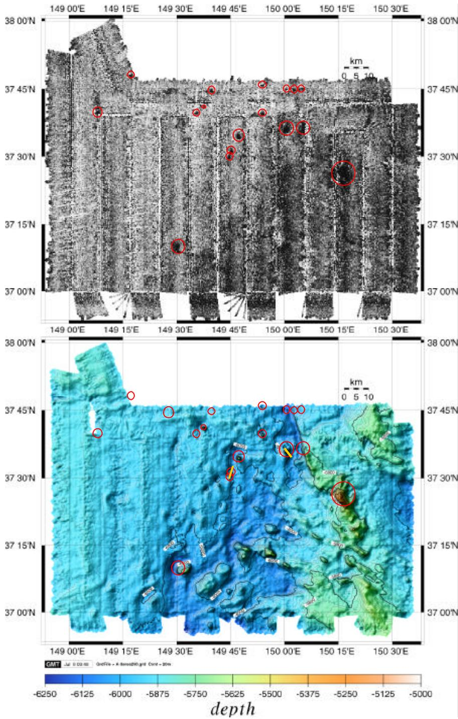
**Figure 2-1-2-1.** The map showing B-area. The bottom and upper figures show the bathymetry and side scan image of this area, respectively.
