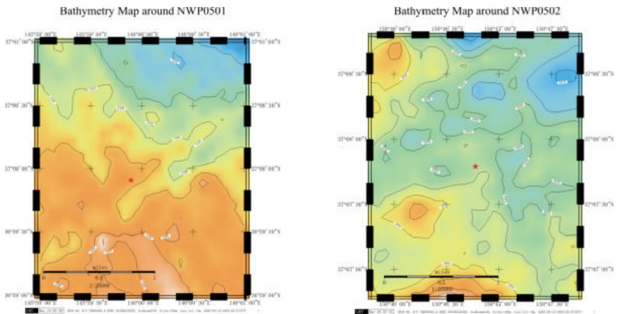
**Figure 5-2-2.** Six OBEM deployed positions superimposed on the bathymetry map revealed by the multi-narrow beam in this cruise.
