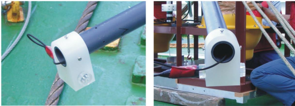
**Plate 4-1-2.** Photograph of the Silver-Silver chloride electrode.
