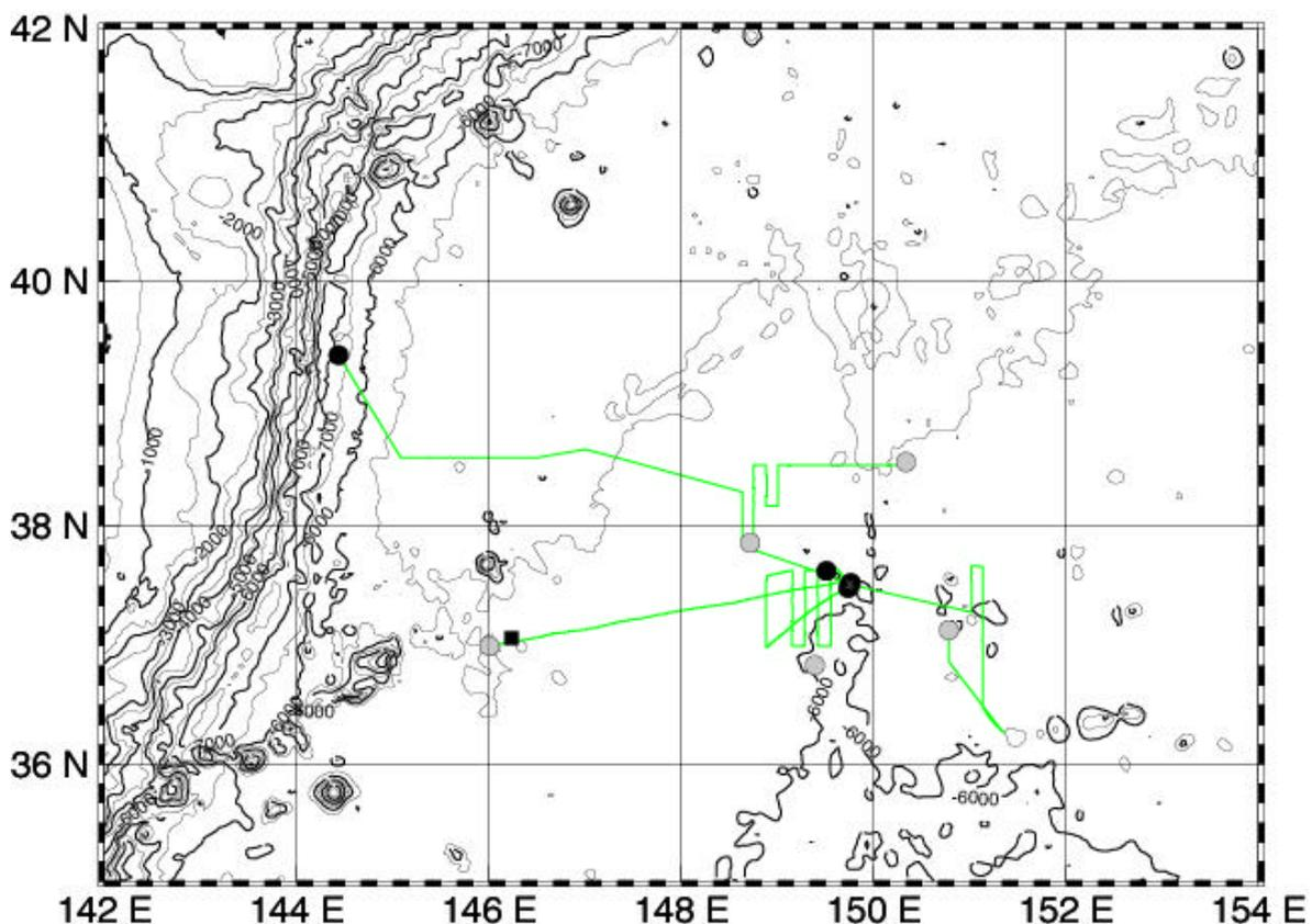
**Figure 5-5-1.** Ship tracks which total force magnetic data were obtained using a proton magnetometer measurement. Vector magnetic data were collected throughout all the survey tracks (See Figure 5-4-1). Black squares indicate locations of "Figure-8 turn". Black circles show Shinkai 6500 dive sites and gray circles show OBEM stations.
