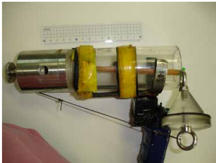
Fig. Before using. The lid is open and connected with the trigger.
