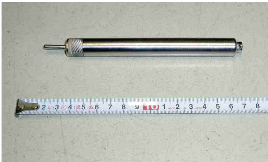
Photo 3-2-2.2. ANTARES Miniaturized Temperature Data Logger (MTL).
