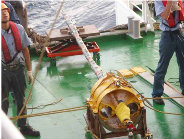
Photo 3-2-2.1. The heat flow probe.
