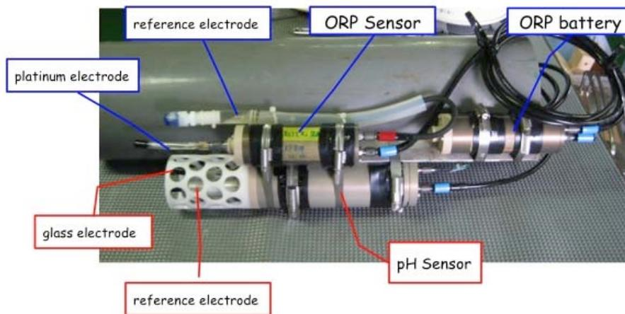
Fig. 5.5 ORP and pH sensor (ORP-08 and pH-08)
