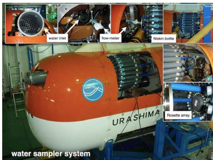
Fig. 5.8 water sampler
