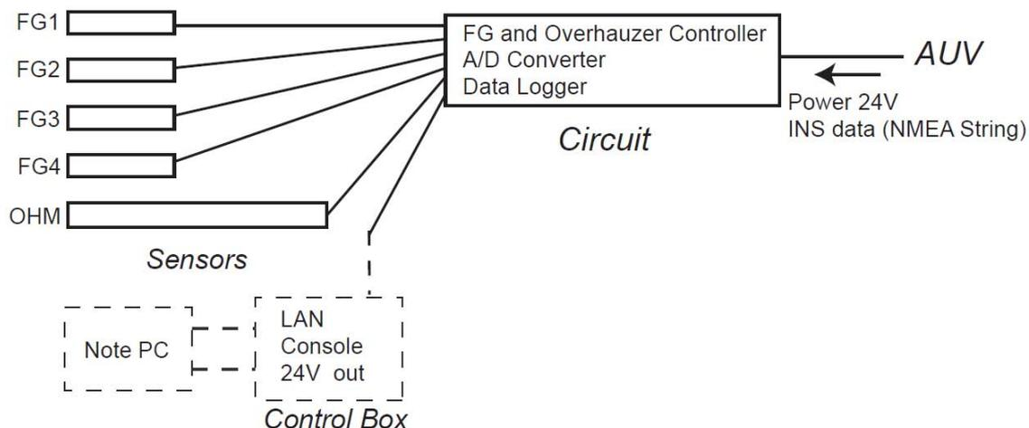
Fig. 5.2. System configuration. Note PC and Control Box are connected for transferring data from data logger to Note PC. FG denotes fluxgate magnetometer sensor and OHM indicates Overhauser magnetometer sensor.
