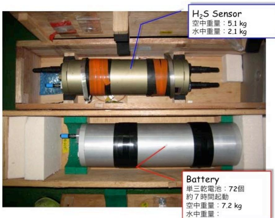
Fig. 5.7 Hydrogen sulfide sensor (H<sub>2</sub>S07) and battery unit.
