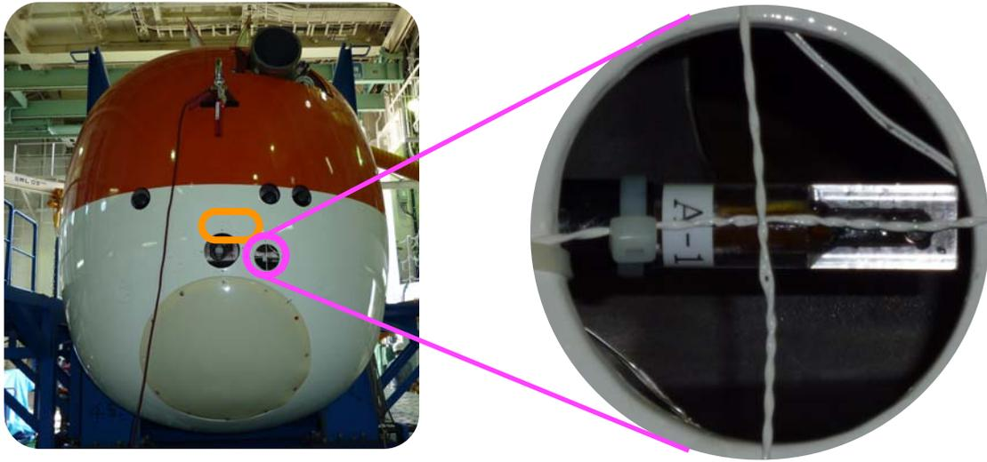
Fig.5.4 ISFET pH sensor equipped on AUV *URASHIMA*
