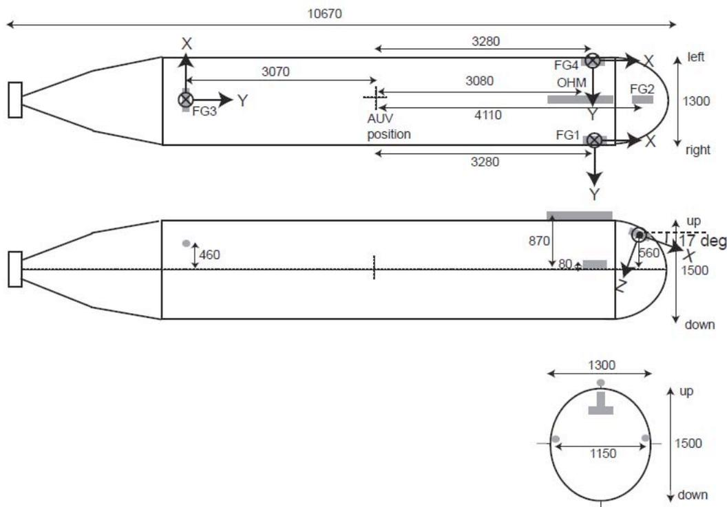
Fig. 5.3 The positions of magnetic sensors and three axis (X-Y-Z) coordinates of fluxgate type magnetometer. Scale unit is in mm.
