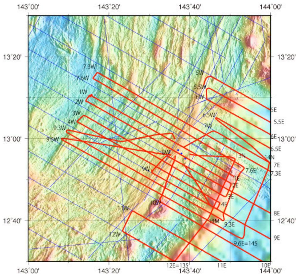
waypoints are shown in Fig.6.1. All lines are perpendicular to the backarc ridge except for two lines parallel to the arc. Sea state was well through the survey. Navigation data were imported from ship's GPS.
