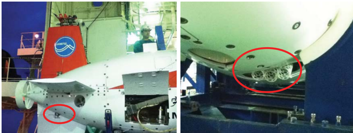
Fig. 4.3.5 Geochemical sensors installed on Urashima
