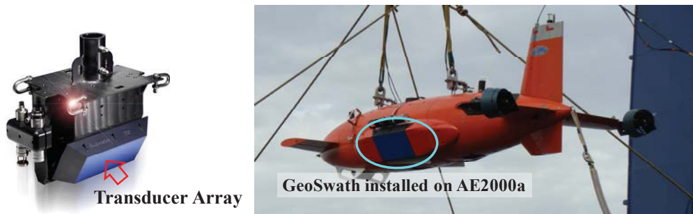
Fig. 4.1.2 GeoSwath system: stand alone (left) and installed on AE 2000a (right)
