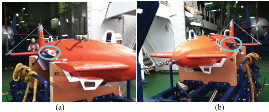
Fig. 4.3.3 Geochemical sensors installed on AE2000a. (a) pH and Turbidity sensor (b) CTD Data logger on left side
