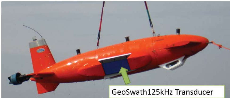
Fig. 6.1.1 GeoSwath transducers mounted on AE2000a platform
