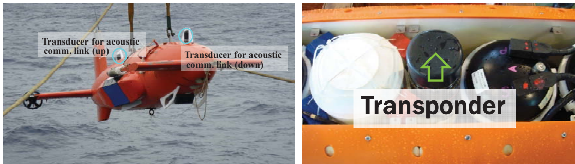
Fig. 4.1.5 Acoustic devices installed in Aqua-Explorer 2000a
