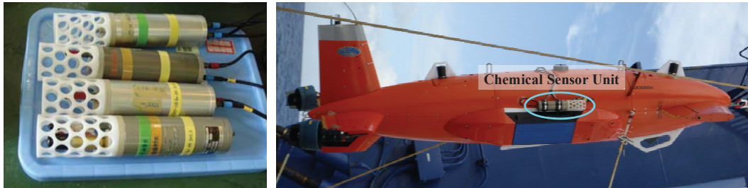
Fig. 4.1.3 Chemical sensor units: stand alone (left) and installed on AE2000a (right)
