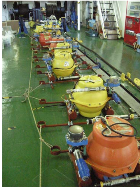
Fig. 5.3.1. Ocean-bottom seismometers on the deck.
