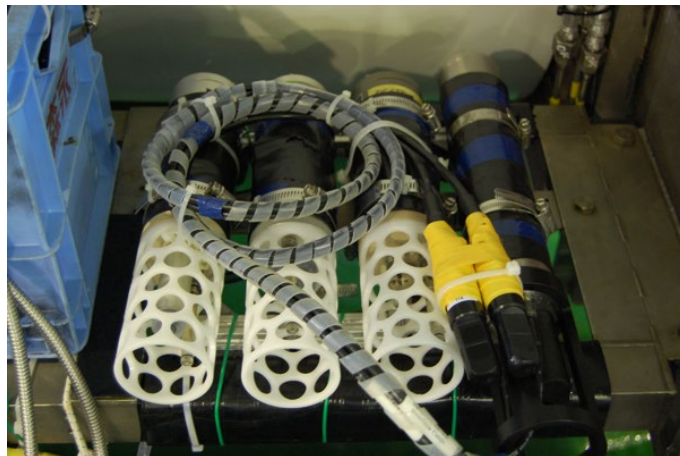
Fig. 5.2.2 pH, ORP and H 2 S sensor with CTD-T profiler mounted on SHINKAI 6500
