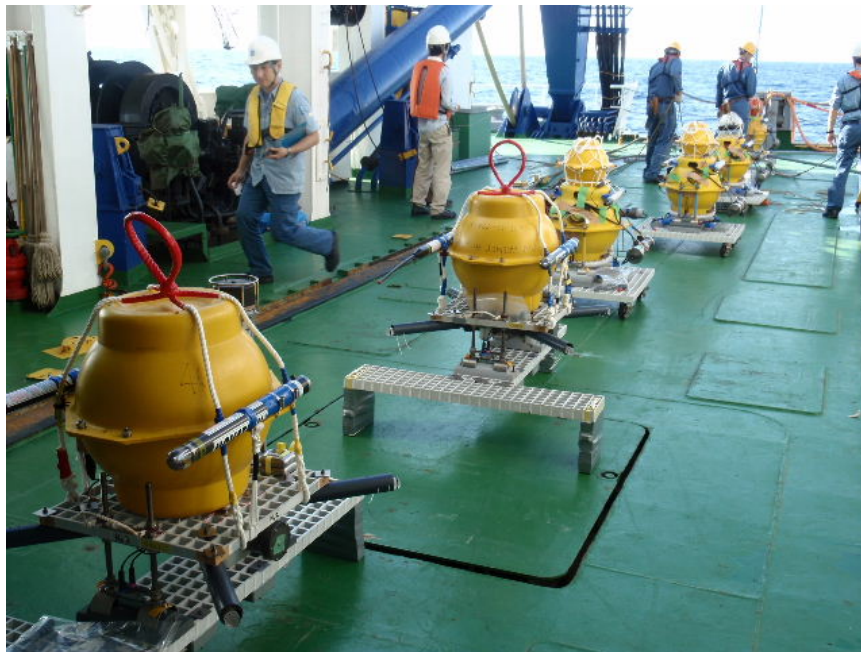
Fig. 5.1.5. Four OBEMs (ocean bottom electromagnetometers) and two OBEs (ocean bottom electrometers) before the deployment (April 27).
