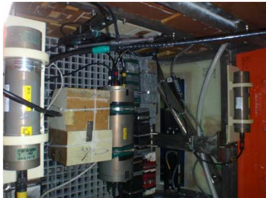
Figure 4: magnetometers in the payload space
