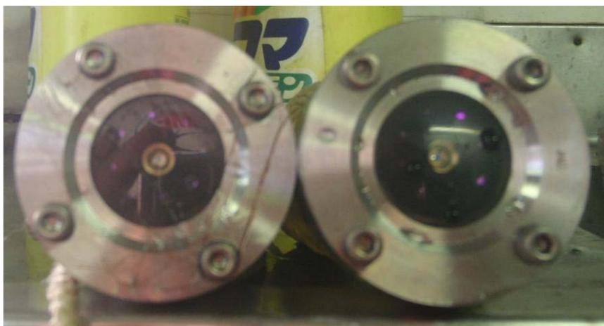
**Figure 7: spider-net-like material adhered on the window of left-handed turbidity meter**
