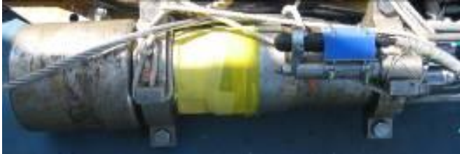
Figure 5.11. Air-gun (left) and single channel hydrophone streamer cable (right)
