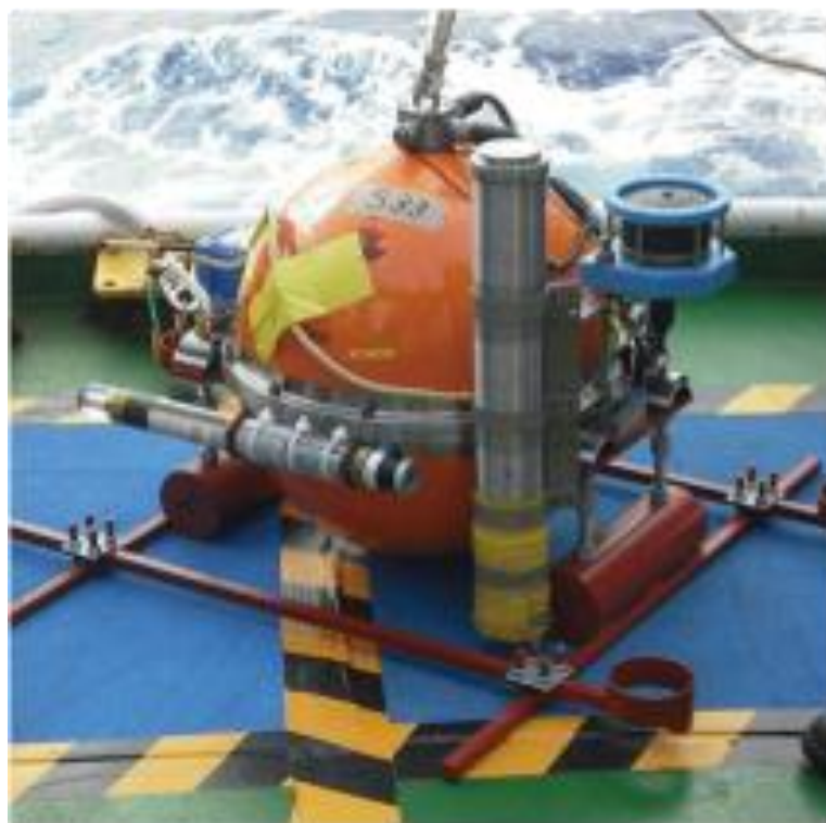
Figure 5.10 OBM (titanium cylinder) attached vertically to titanium sphere OBS.
