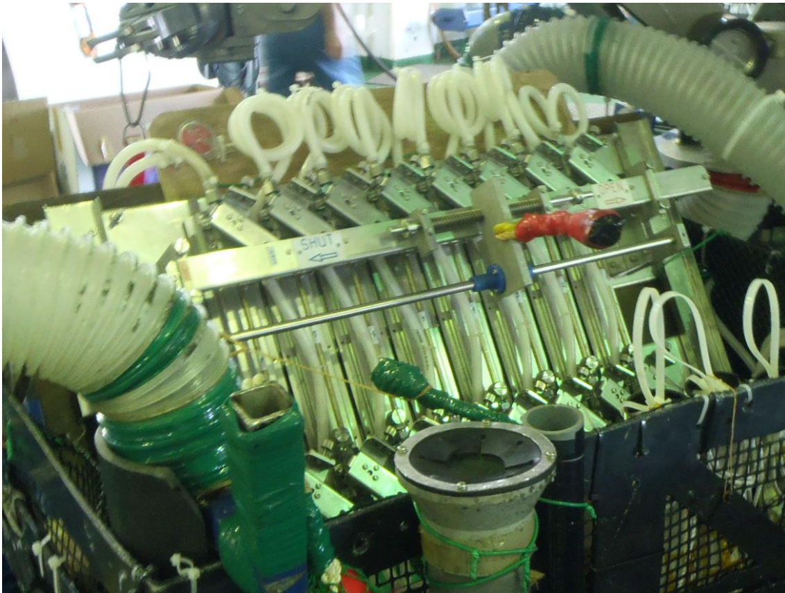
Figure 5.3. Ore-type 8-fold fluid sampler attached to Shinkai 6500.
