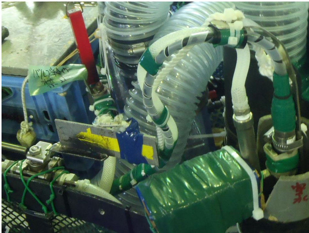
Figure 5.4b. Suction sampler with small canister attached to Shinkai 6500.
