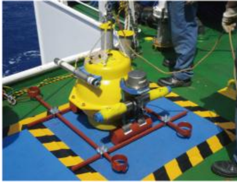
Figure 5.8b. OBS (glass sphere)
