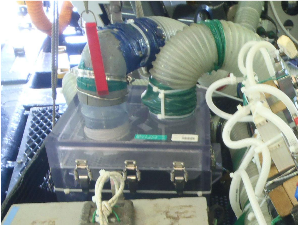
Figure 5.4a. Suction sampler with large canister attached to Shinkai 6500.
