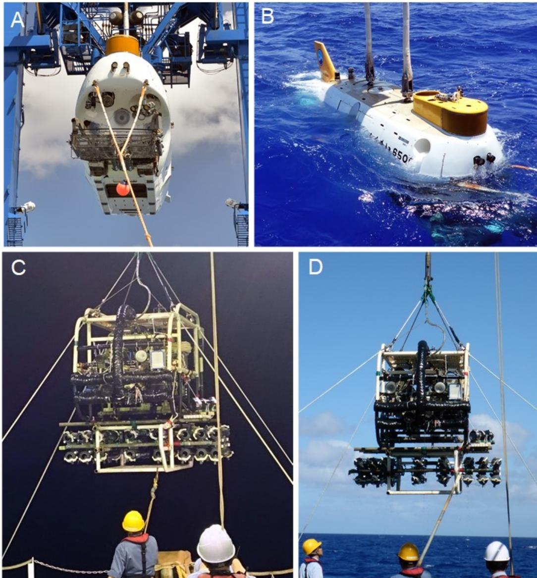
**Figure 7.** The Shinkai 6500 submersible (A, B) and the YKDT towed camera system (C,D) being deployed during the YK17-10 cruise in May 2017. Both underwater observation systems had multiple camera systems, and Niskin water collection bottles were attached to collect water samples.
