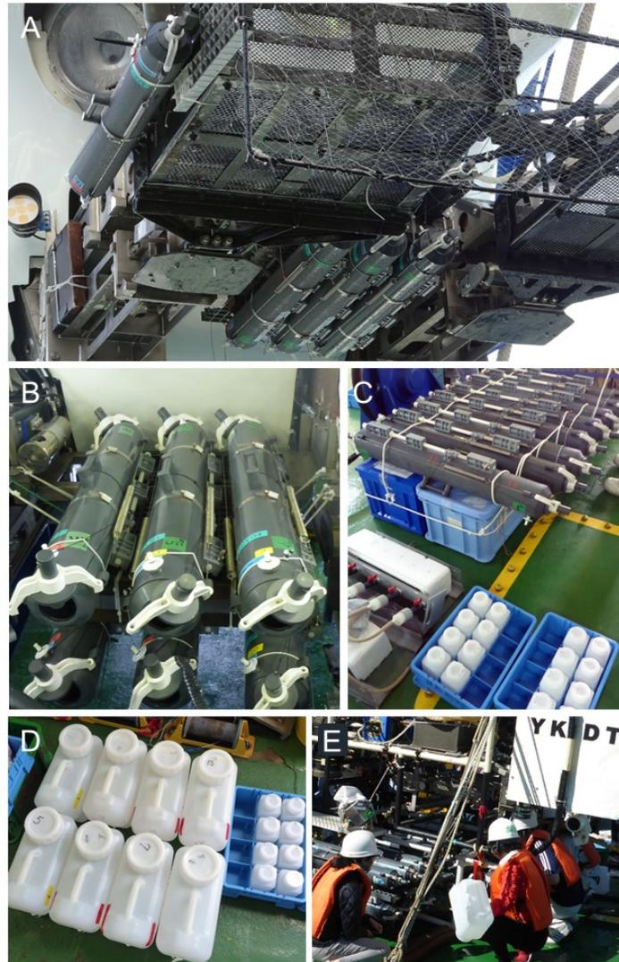
**Figure 9.** Locations of the Niskin bottles on the front and side of the Shinkai 6500 submersible (A, b), the bottles arranged in preparation for collecting water samples for filtration (C), the large bottles used to collect water samples for eDNA filtration and the small bottles for amino acid analyses (D), and water samples being collected from the YKDT Niskin bottles.
