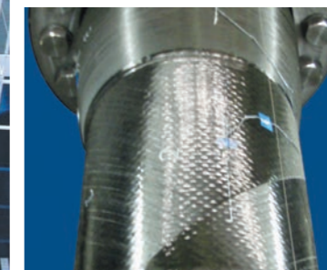
Left: A contemporary steel riser pipe. Above: CFRP riser pipe with carbon fibers (in development).
