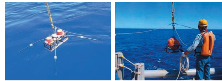
An ocean-bottom-electromagnetometer (OBEM, left) and ocean-bottom seismometer (OBS, right) being deployed to the ocean floor.
