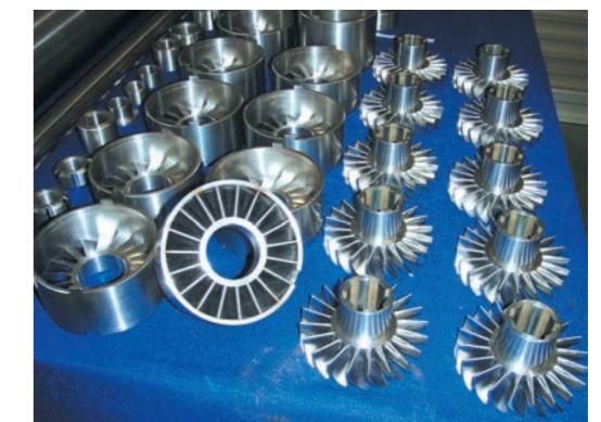
Above: Mud driven turbine motor to be incorporated in the coring system. Below: Rotors and stators of turbine motor.
