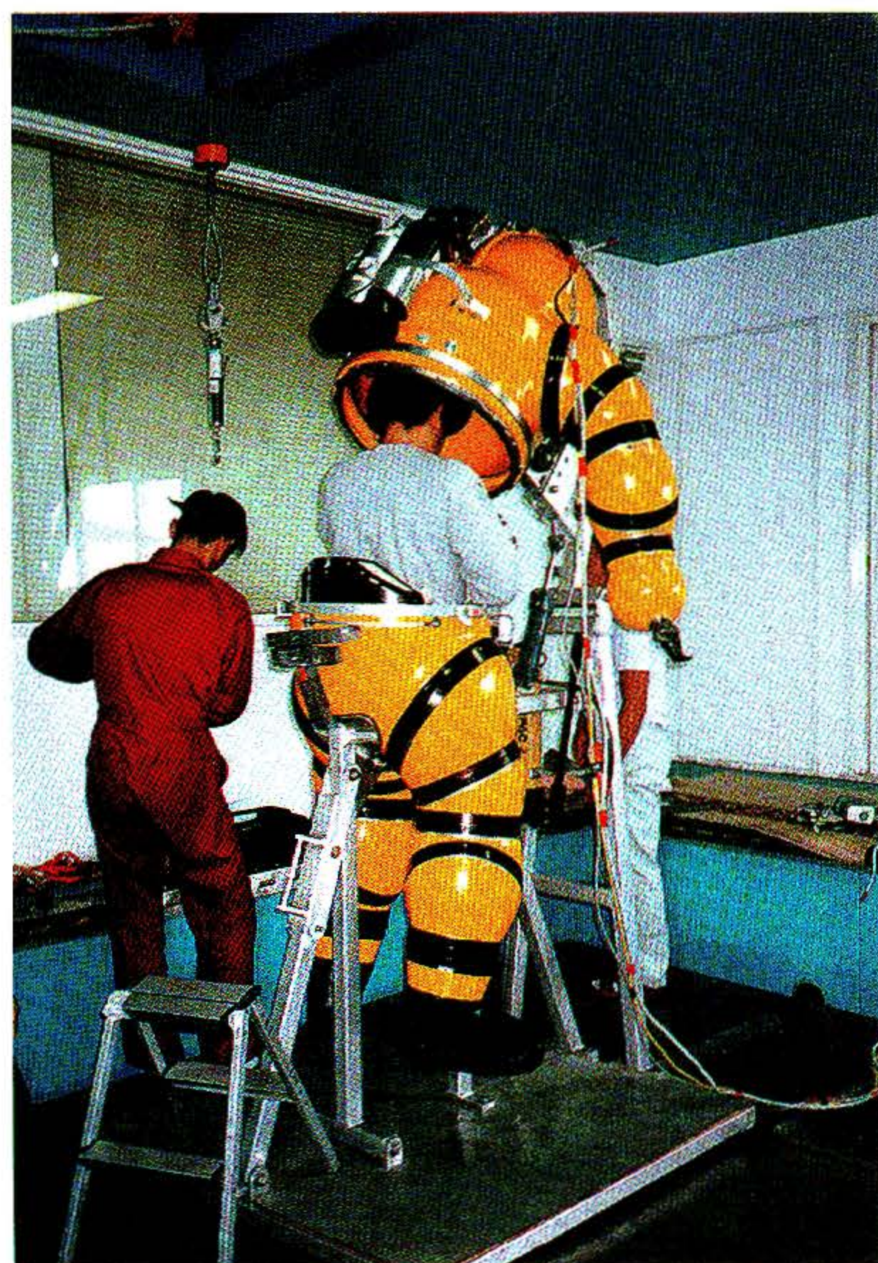
写真3 大気圧潜水服の着脱（歩行型） Photo 3 Newtsuit walk-type (without thruster pack), the upper part is separated at the waist joint.
