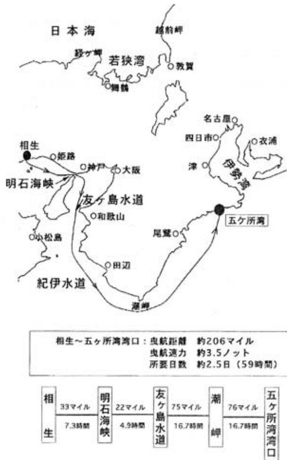
図13 曳航経路 Fig. 13 Towing route
