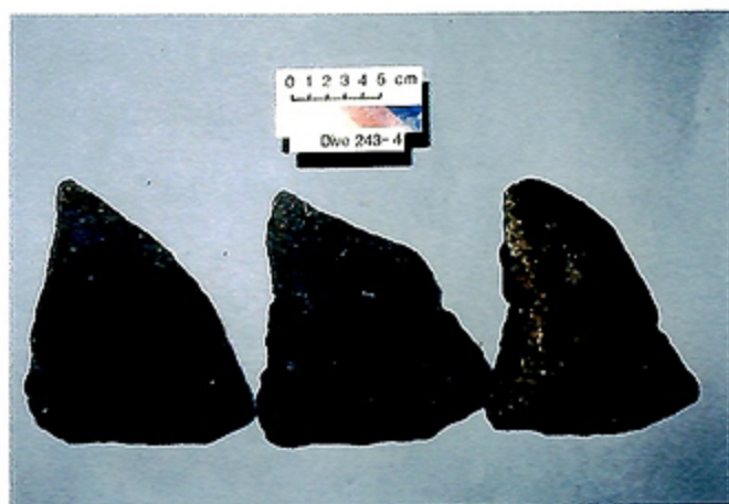
写真7 安山岩 (243-4) の表面 (右) と切断面 (左と中央) Photo. 7 Andesite (243-4): appearance (right) and cut sections (left and center).
