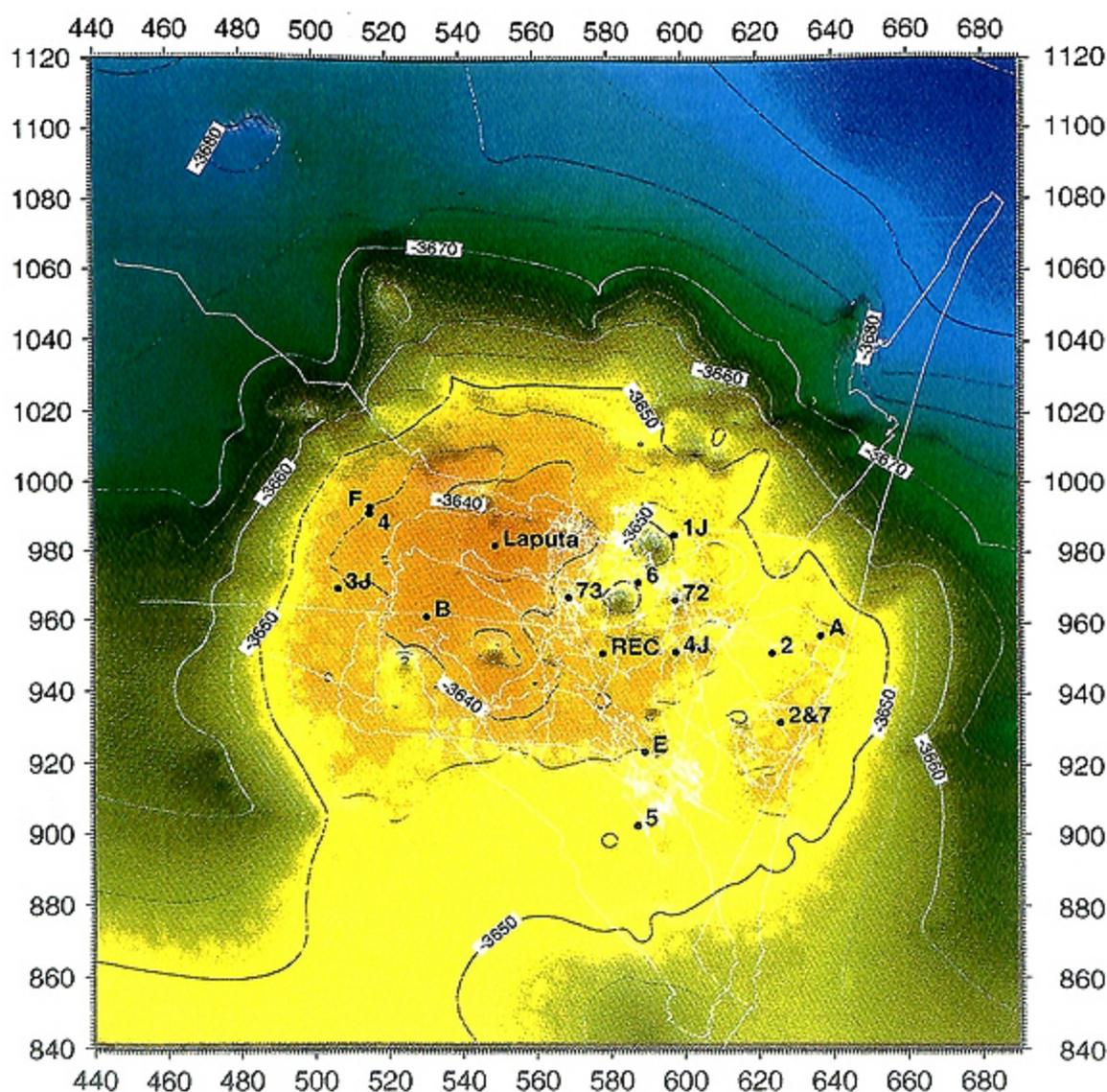
Figure 2 Bathymetric map of the TAG hydrothermal mound. Markers from A to E were deployed by Alvin; Markers 1J to 4J and 72 to 73 were deployed by Shinkai 6500; Laputa is the central black smoker complex; REC is the ODP Re-entry cone.
