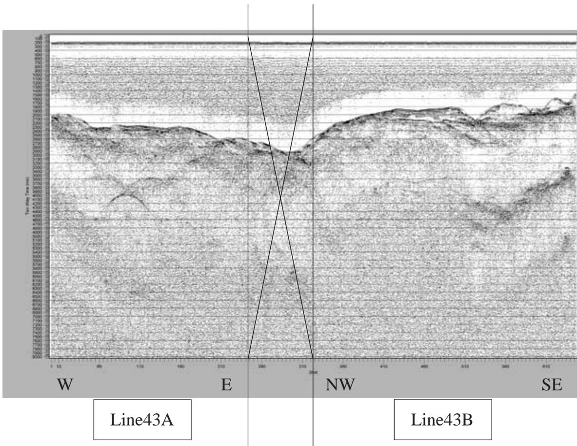
Fig. 3 (Line43AB) Seismic profiles along the survey tracks.
