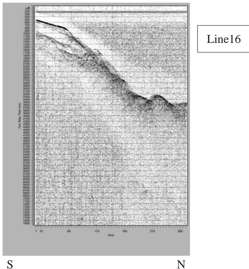
Fig. 3 (Line16) Seismic profiles along the survey tracks.
