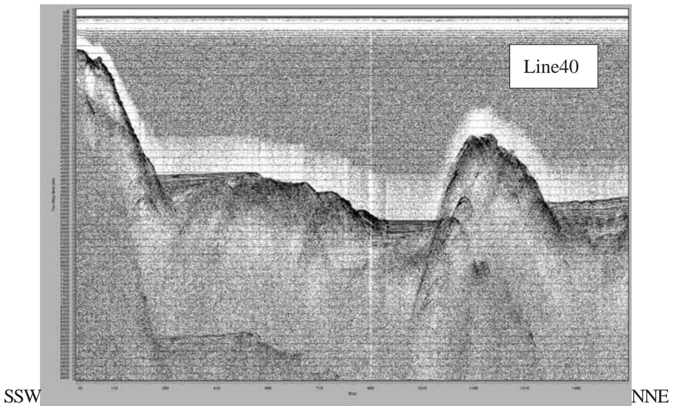
Fig. 3 (Line40) Seismic profiles along the survey tracks.
