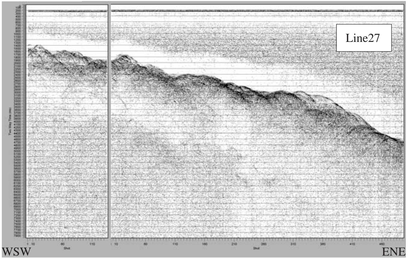
Fig. 3 (Line27) Seismic profiles along the survey tracks.
