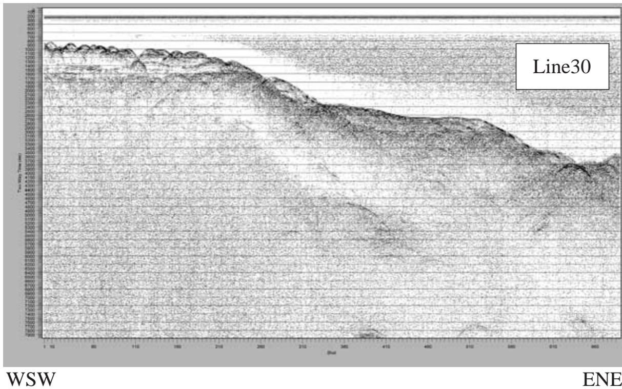
Fig. 3 (Line30) Seismic profiles along the survey tracks.
