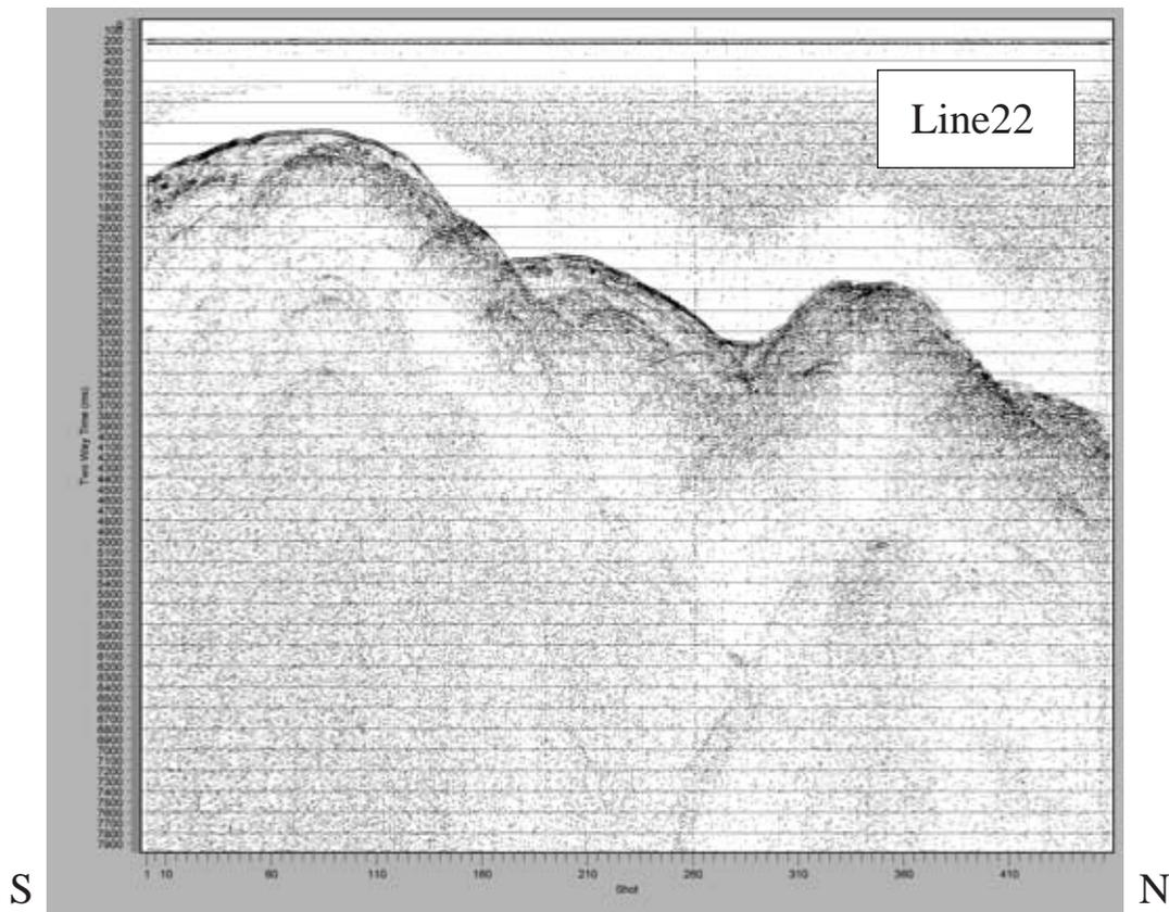
Fig. 3 (Line22) Seismic profiles along the survey tracks.
