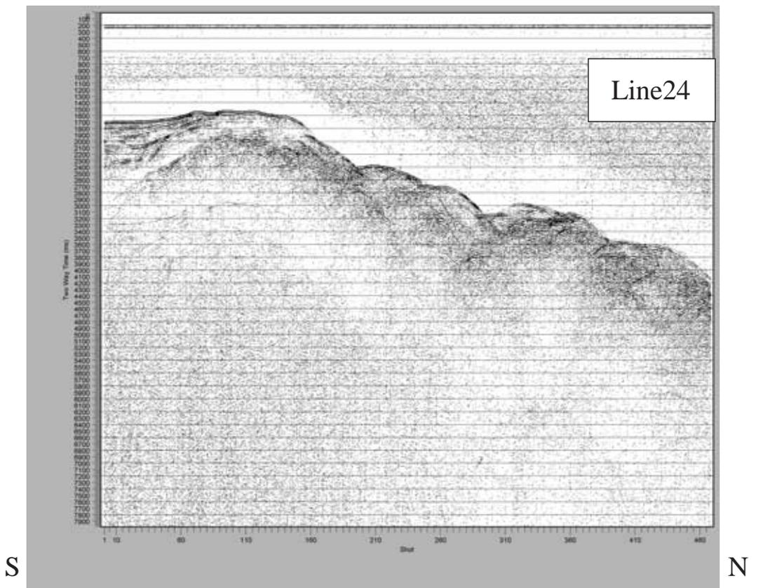
Fig. 3 (Line24) Seismic profiles along the survey tracks.
