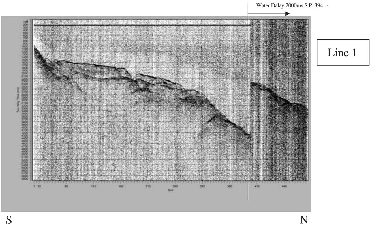
Fig. 3 (Line1) Seismic profiles along the survey tracks.
