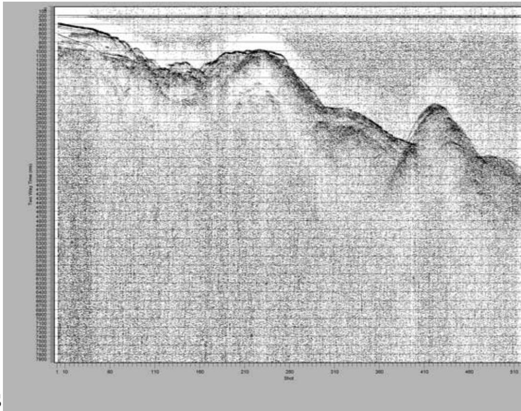
Fig. 3 (Line7) Seismic profiles along the survey tracks.
