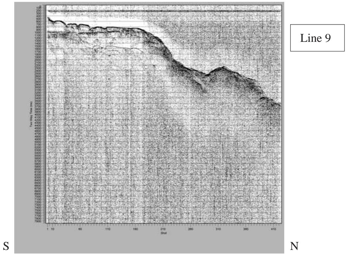
Fig. 3 (Line9) Seismic profiles along the survey tracks.
