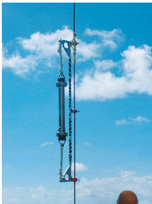
Fig.15 Acoustic unit (so called, "fish") fixed at 100 m above the bottom electrode for positioning the bottom electrode.
