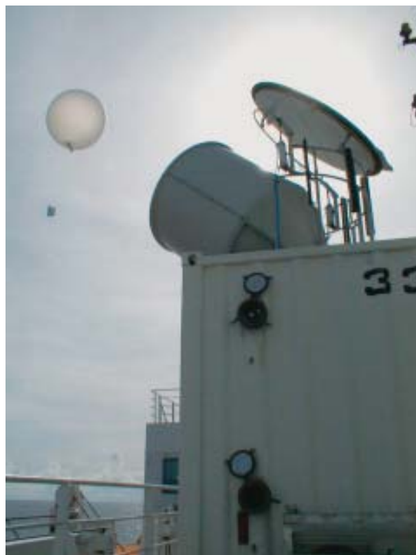
Fig. 1 Launch the radiosonde from container.
