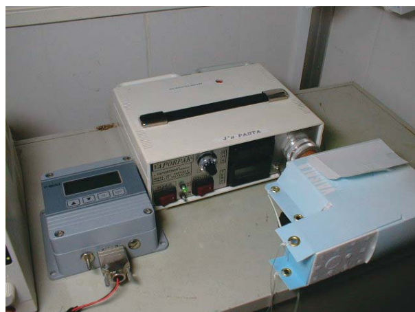
Fig. 5 Sensor calibration prior to launch. Reference barometer (left) and humidity calibrator (center).
