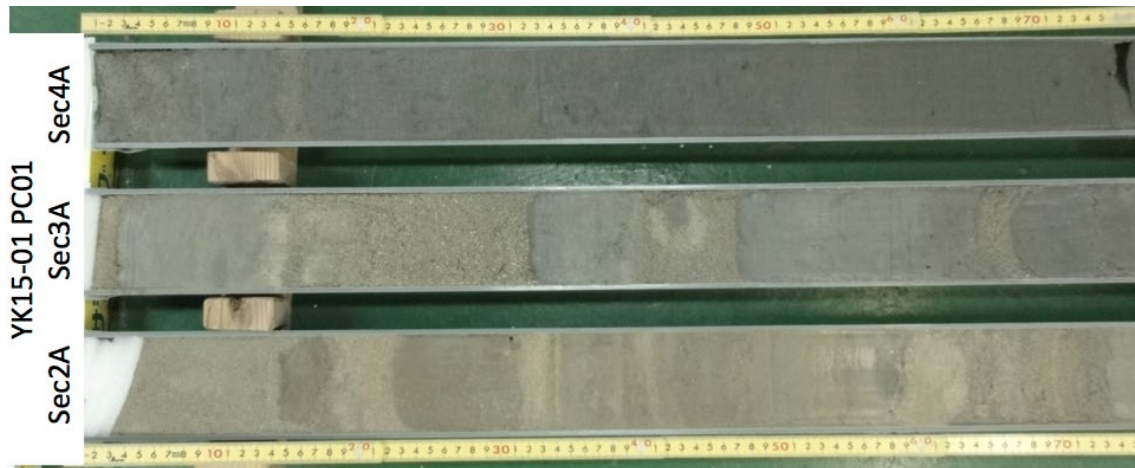
Fig. 2 Photo of YK15-01 PC01 (23-56.3055°N, 124-04.4122°E, 2,765m). Note intervals of light color correspond to turbidites including shell and coral fragments.
