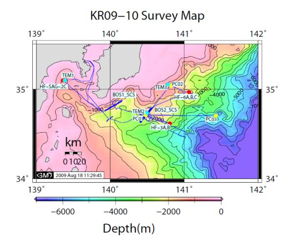
Ship track (blue line) and stations of measurement and sampling on KR09-10 cruise. TEM (blue circles): Installing pop-up water temperature measurement system, HF (red circles): heat flow measurement, PC (yellow circles): piston core sampling with heat flow measurement, SCS: single-channel seismic survey.
