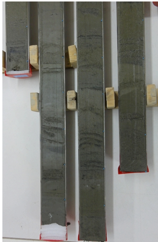
Fig.2: Frequent occurrence of turbidite layers observed in PC21 (core diameter = ca. 74mm)
