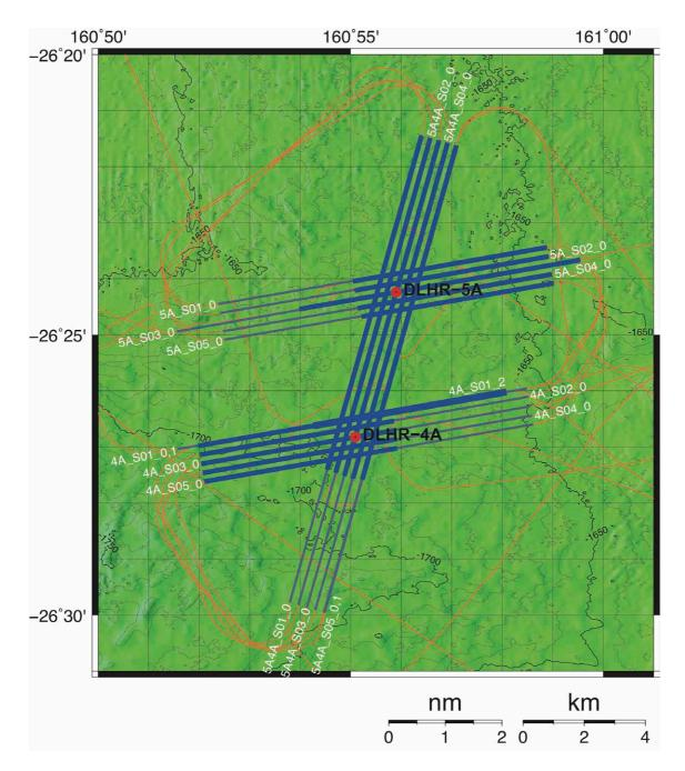
Figure 10. HR-MCS survey lines in the DLHR-5A/4A area. Blue thin and thick lines indicate regions of air gun shooting with partial volume and full volume, respectively. R/V Kairei's track during the OBS-MCS survey is shown by the orange line.
