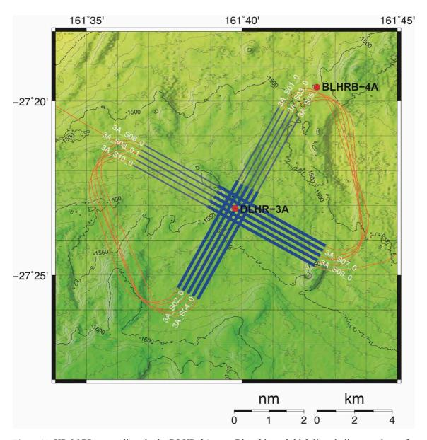
Figure 11. HR-MCS survey lines in the DLHR-3A area. Blue thin and thick lines indicate regions of air gun shooting with partial volume and full volume, respectively. R/V Kairei's track during the OBS-MCS survey is shown by orange line.
