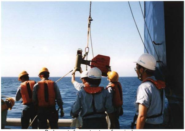
Deployment of current meters of mooring buoy
