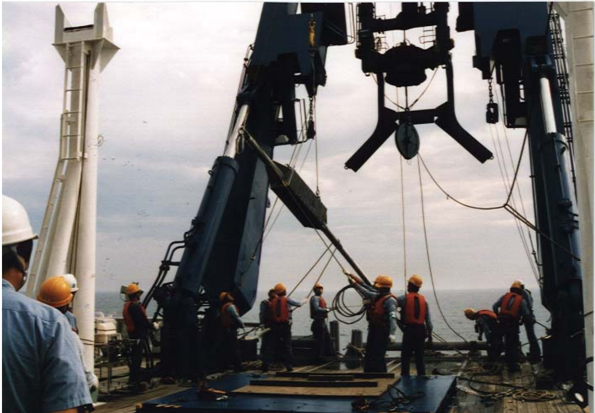
Piston corer (large diameter:115m)
