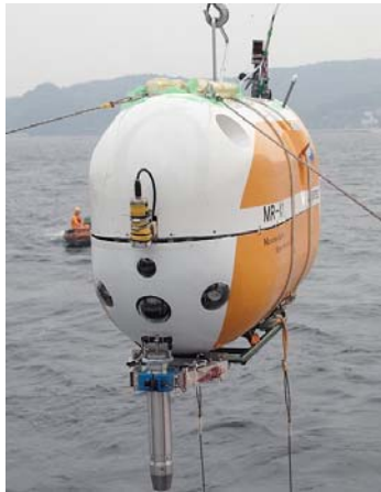
Fig. 6 : The MR-X1 with the mud sampler (left) and the cesium magnetometer (right).
