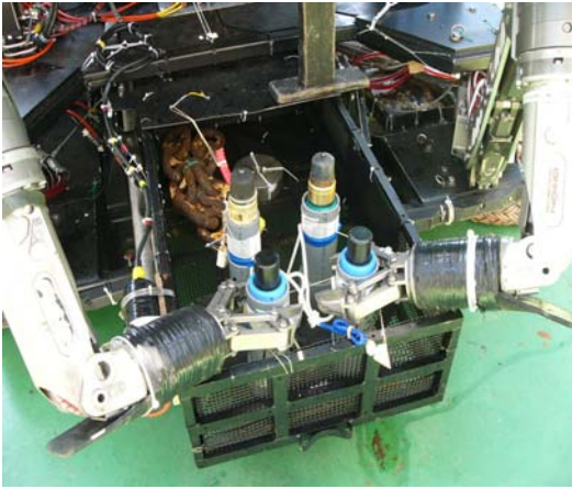
Fig.1 Left: ROV homers. Right : Video image of acoustic survey. The seismometer package is shown in the right of figure, and the submarine cable is also visible behind the ROV homer.
