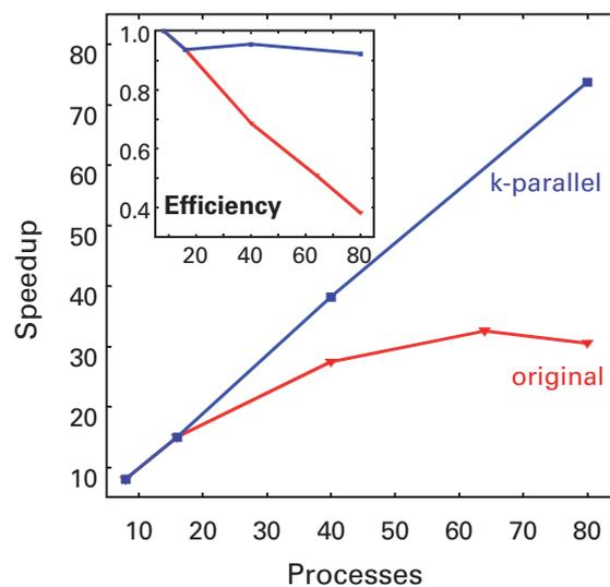
**Fig. 3** Performance of k-point parallelized VASP code.
