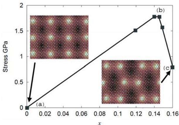
**Fig. 5** Stress-driven instability of dislocation cores: (a) an initial position, (b) a critical position, and (c) a displaced position of the cores. The parameter  $x$  corresponds to the shear strain  $\gamma_{23}$ . Positions of dislocation cores are seen as highlighted atoms in the inset images.
