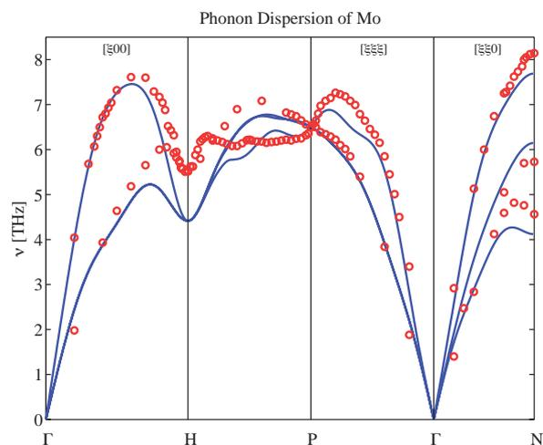
**Fig. 2** Phonon dispersion curve of BCC Mo 250 atoms with  $6 \times 6 \times 6$  k-points (lines) compared with the experimental data [7] (open circles). The detailed structure near the H point has been reproduced.
