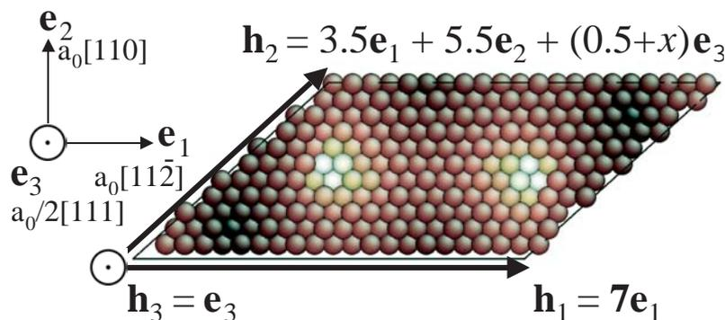
Fig. 4 The BCC Mo supercell consisting of 231 atoms.
