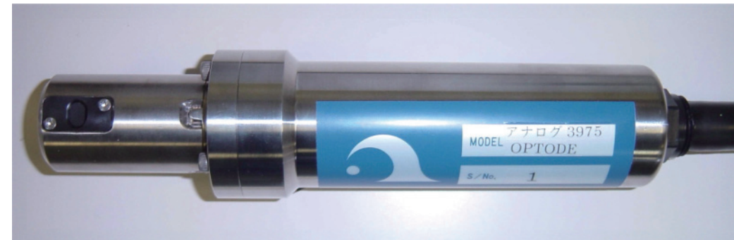
Figure 3.1.6. Oxygen Optode (3830) with analog adaptor (3966). The analog adaptor is packed into titanium housing made by Alec Electronics Co., Ltd.
