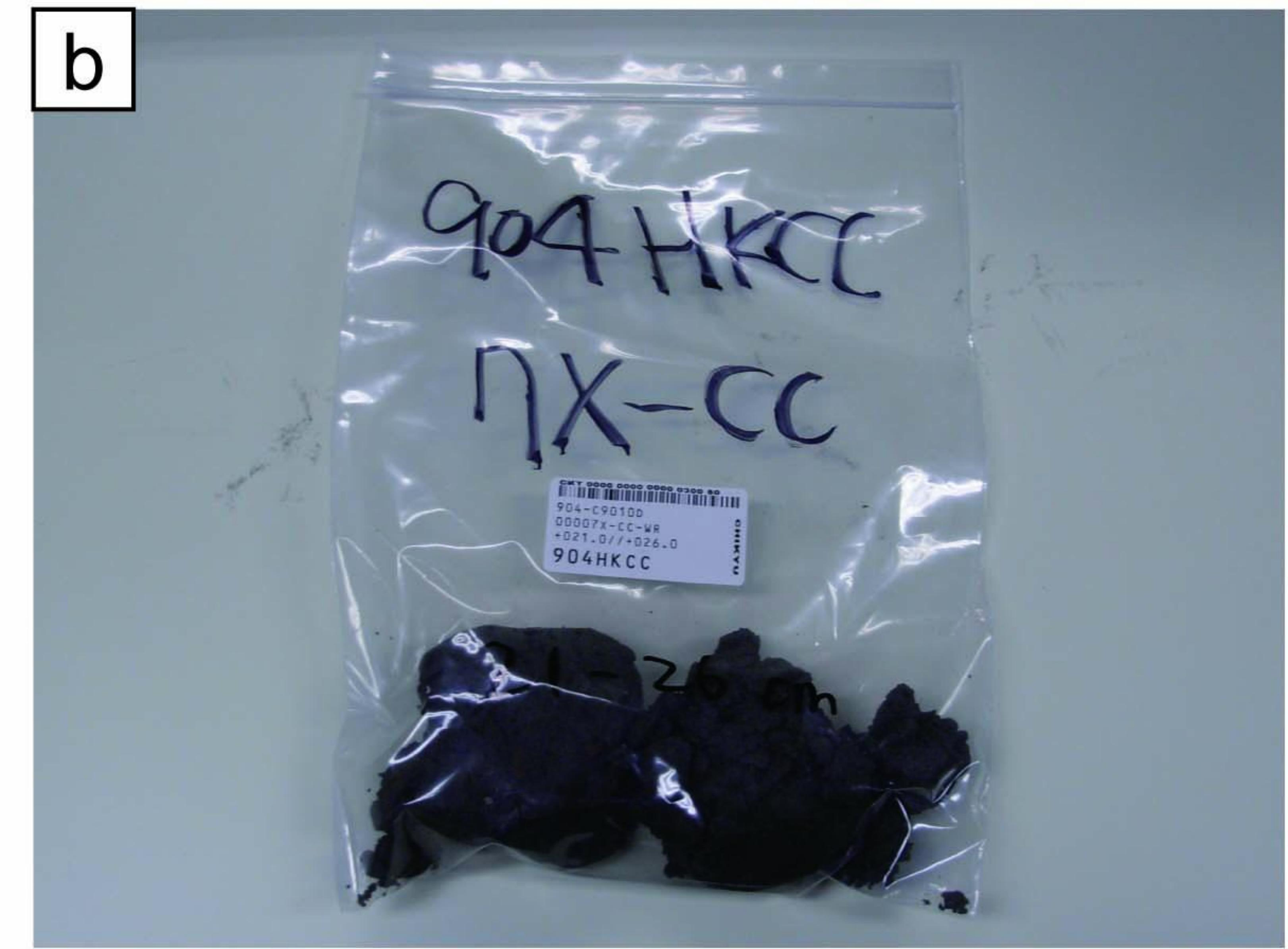
Fig. 6-7-2: 904HKMC: the cubed samples from the working halves. The plastic cubes (a) were plugged in (b, right cube) and out with a hook-like spatula (b, left cube). Each cube was labeled and fully sealed up (c) and zipped (d).
