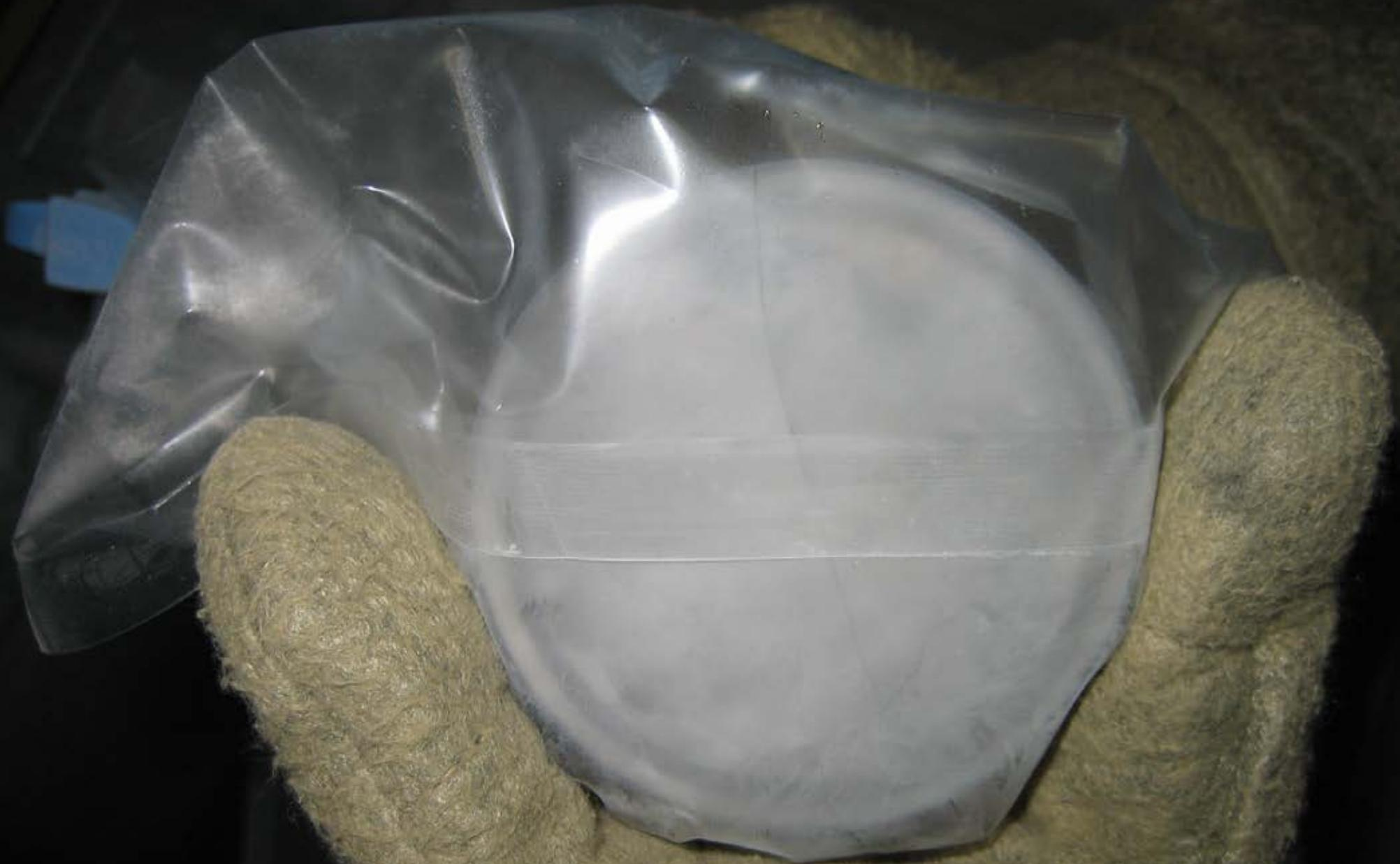
Fig. 6-6-7: Plastic bags containing suspension of fluorescent microspheres, attached on spacer.
