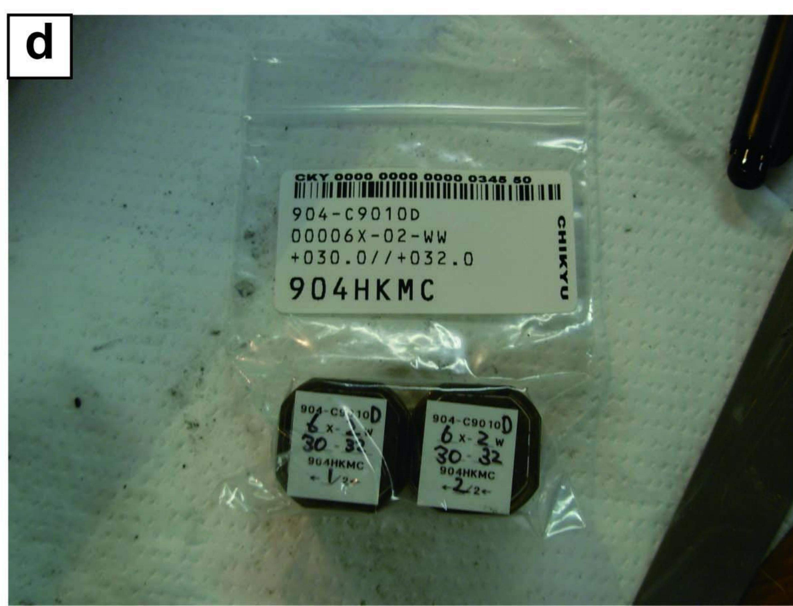
Fig. 6-7-3: 904HKMH: the half round core samples. The samples were taken with a stainless steel scoop for quarter round sampling (a). The rim of the sediments was swept out with a spatula with notches (b and c). These samples were packed in plastic bags (d).
