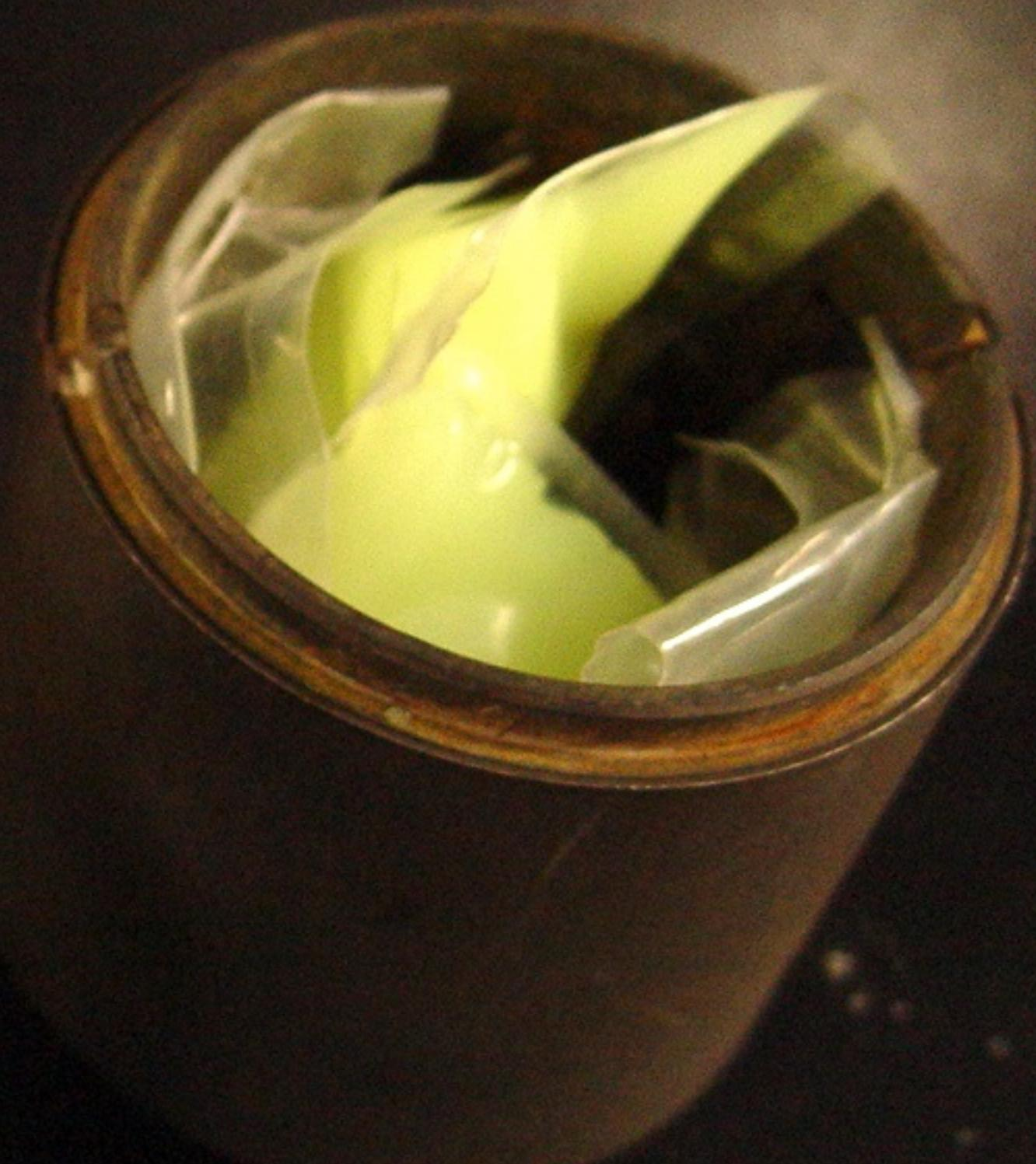
Fig. 6-6-8: Broken plastic bag in recovered cores. (a) Above the core liner of Core 3H. (b) Above the core liner of Core 4H. (c) Lower part in the core liner of Core 4H.
