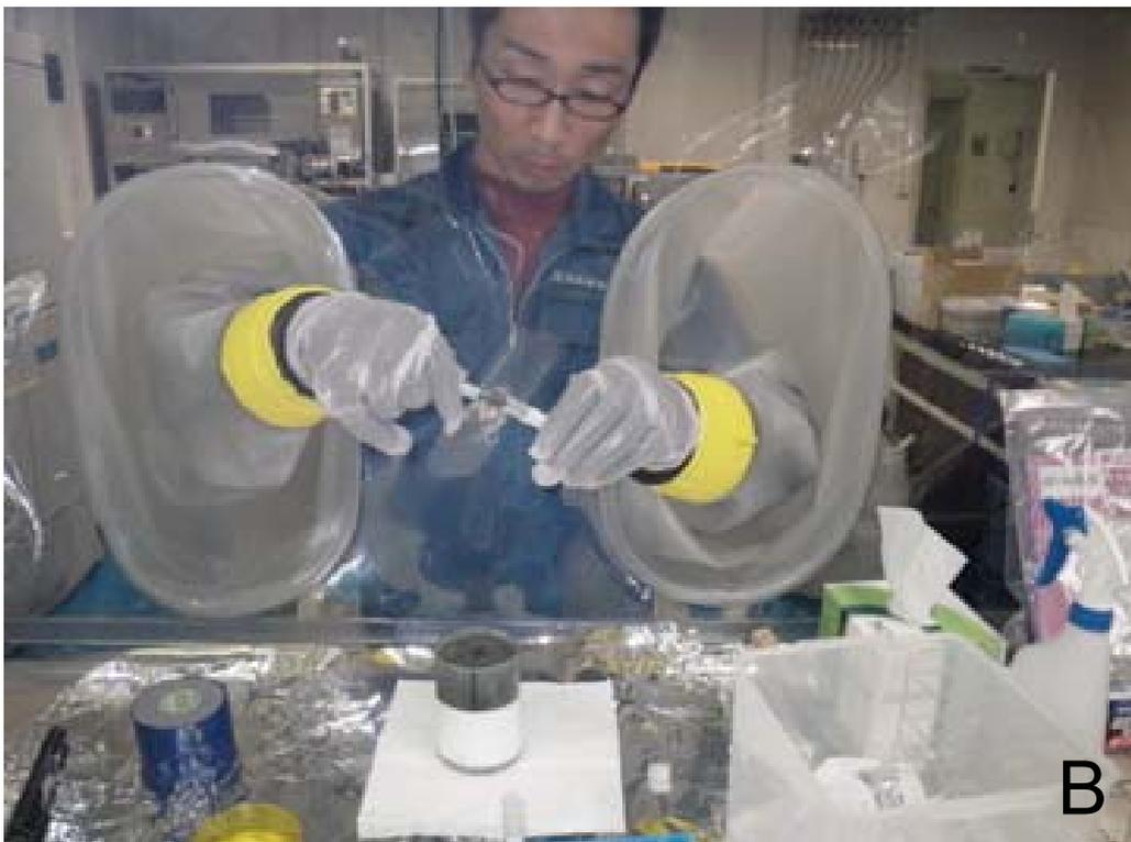
Fig. 6-7-3 We carried out sub-sampling in an aerobic chamber. Insert tip-cut 30 ml syringe into a WR core from the top (A), sub-samples are also taken from syringe sample (B)
