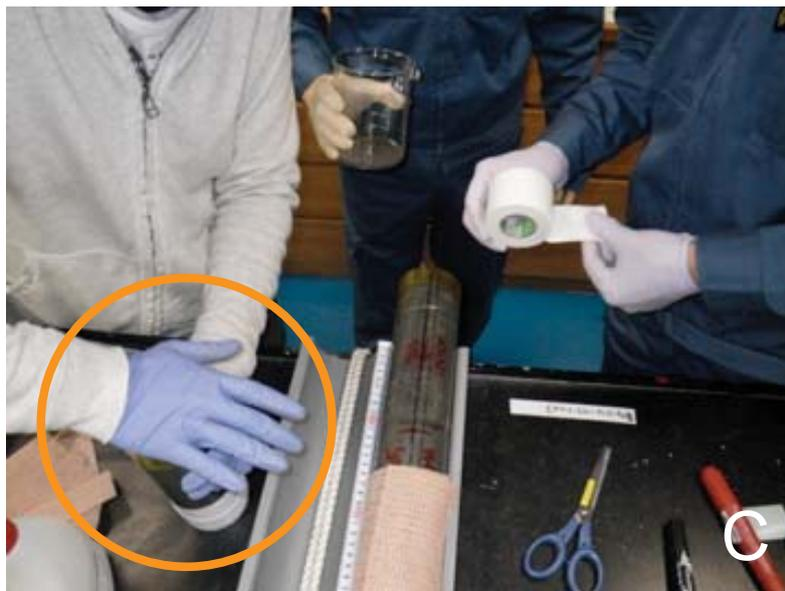
Fig. 6-7-1 WR core sampling. WR cores are cut with rotary core cutter (A), WR cores are sliced with EtOH-sterilized spatula (B), and then capped with yellow EtOH-sterilized end-caps (C).
