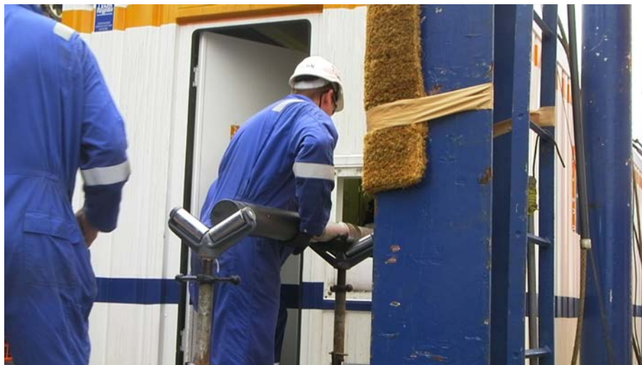
Fig. 6.7.1. Transfer of pressure core into GeoTek PCATS container.
