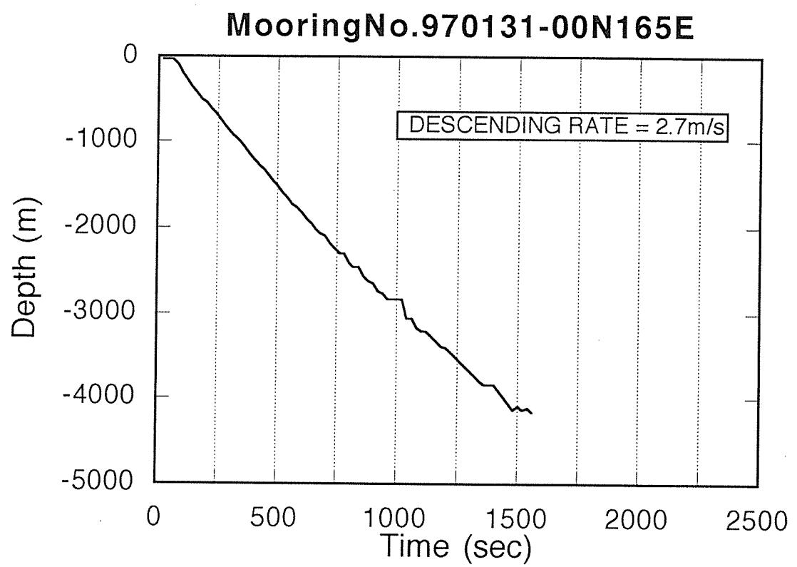
Fig. 7-1 Releaser Depth Monitor
