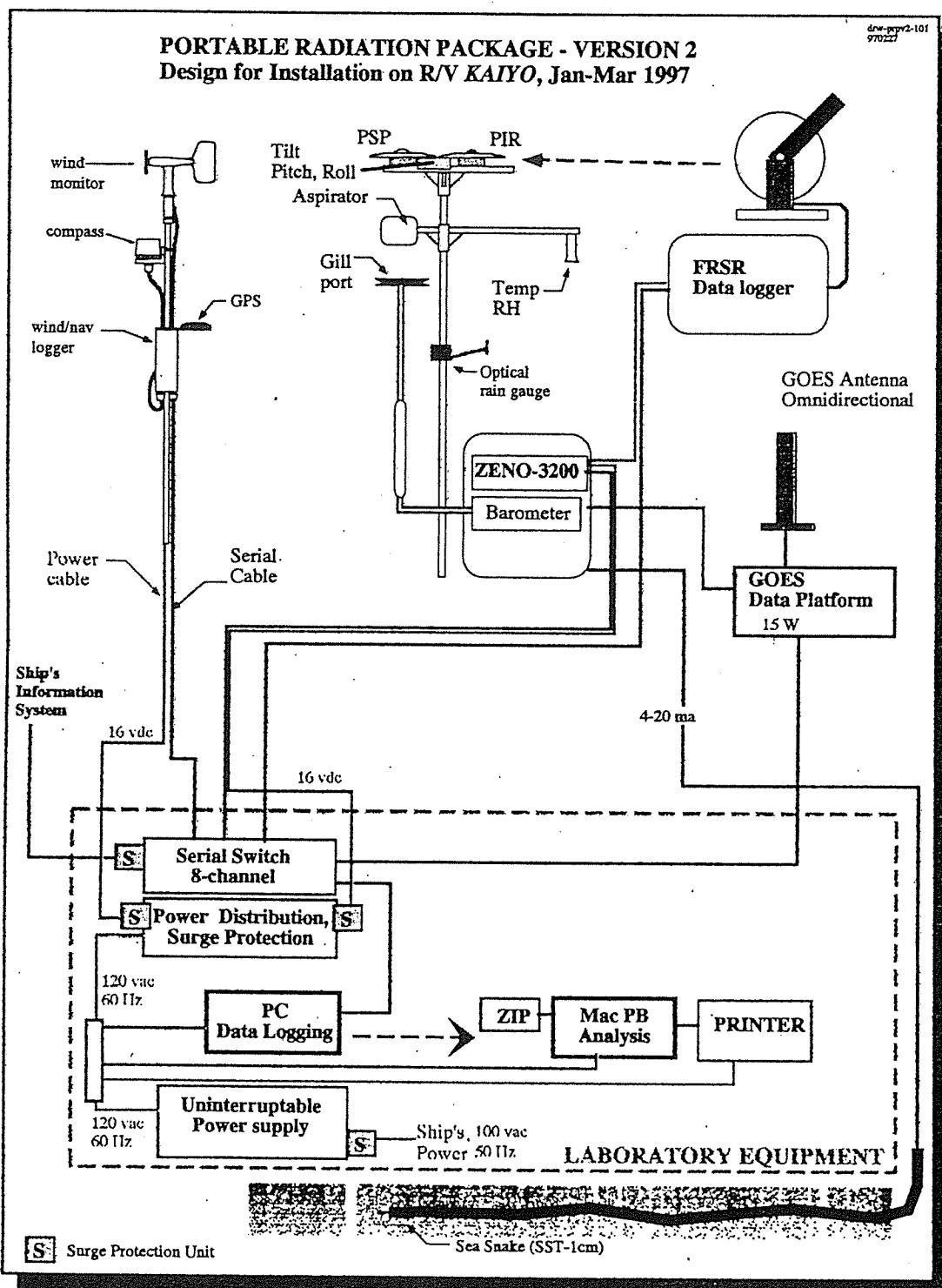
Figure 10: Sketch of the complete JUSTOS mean meteorology flux system. (prpv2-1)
