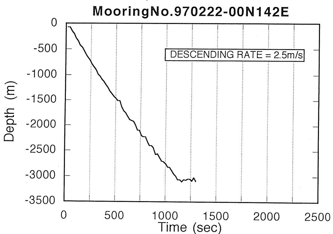
Fig. 7-3 Releaser Depth Monitor
