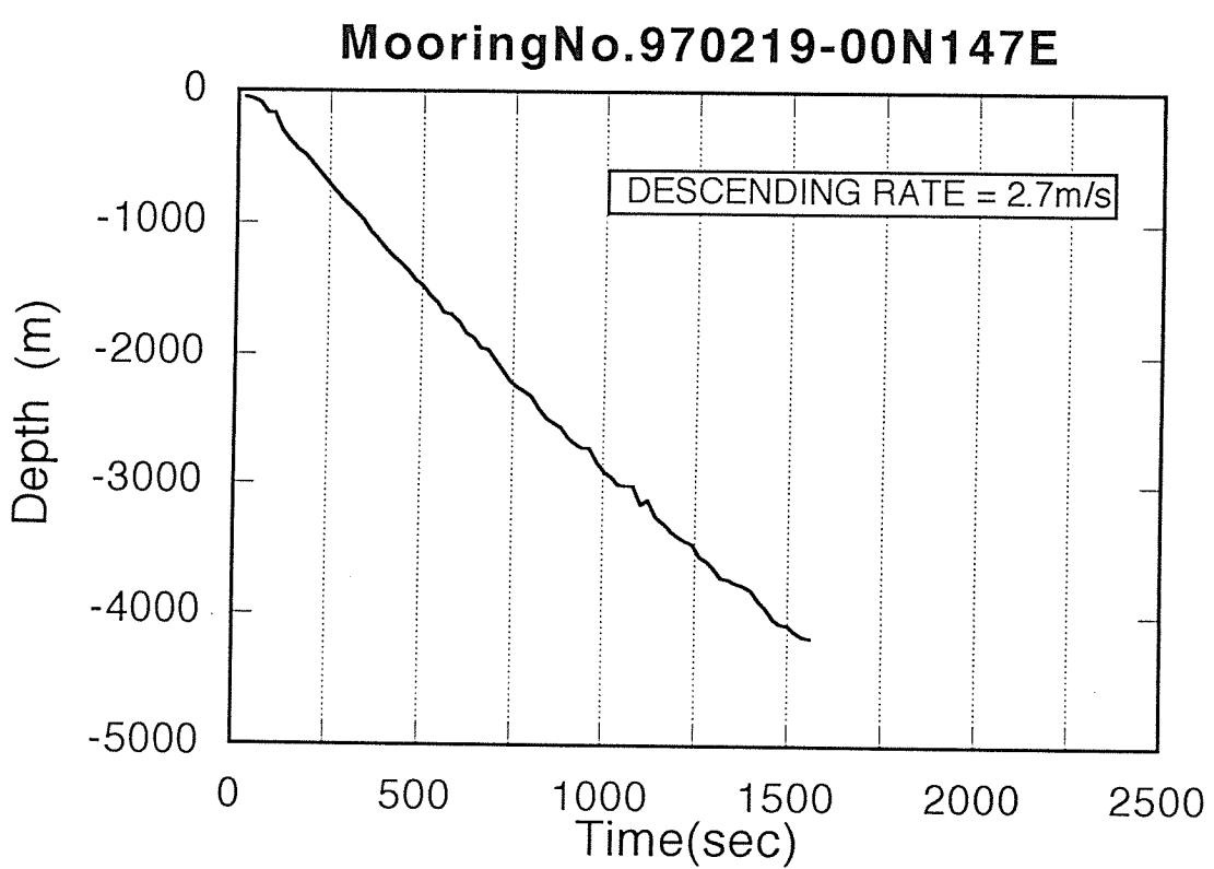
Fig. 7-2 Releaser Depth Monitor
