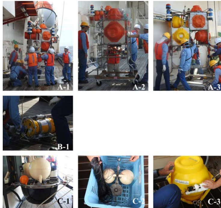
Fig. 3.7-1. Photographs of recovered mooring systems. A-1, A-2, A-3: Lander moored at Sta. M-2, M-3 and M-4, respectively B-1 : ADCP C-1, C-2, C-3: Top buoy, launcher of SEASAW, and sensors of glass sphere.
