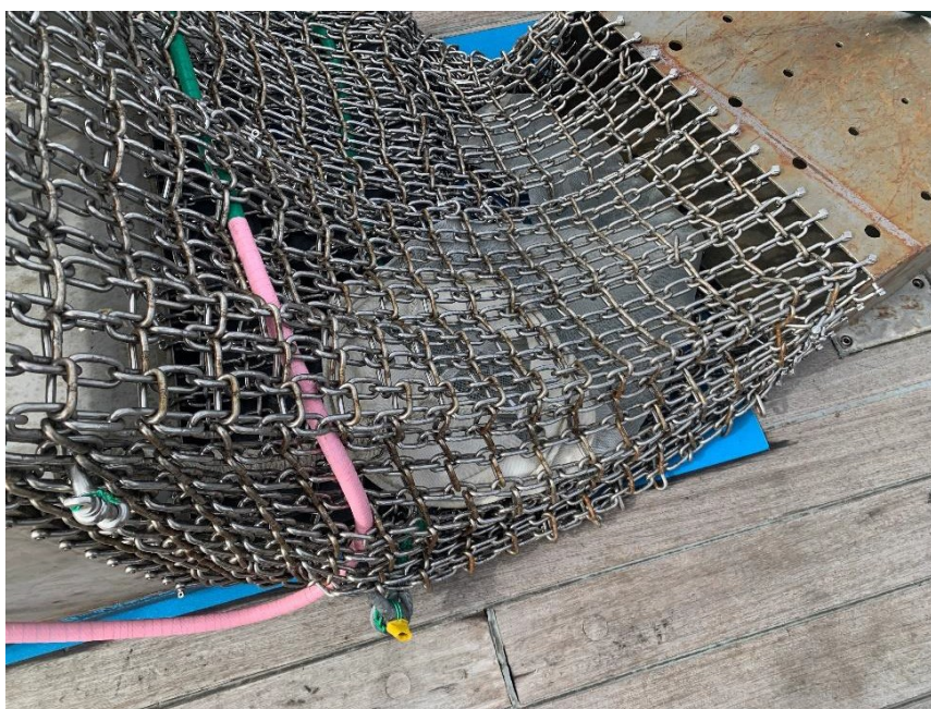
Figure 18. Nylon mesh bag installed in the Gyaico-type dredge for benthos sampling.
