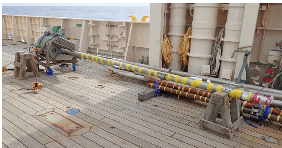
Figure 3.3-2. ANTARES Miniaturized Temperature Data Logger (MTL).
