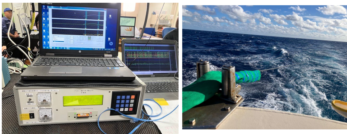
Figure 5(a) left: proton magnetometer and logging computer (Lab-3), (b) right: sensor towed behind the ship.
