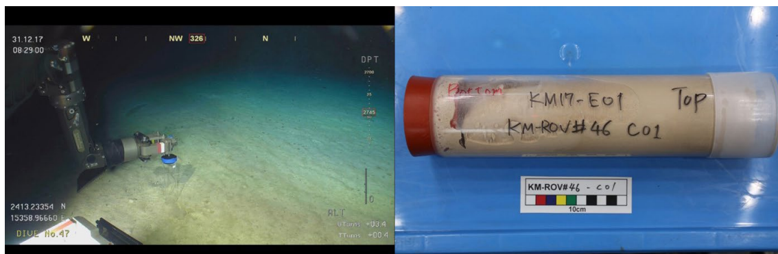
Figure 16. Sediment cores of the length of ~30 cm were collected from the same area where SAHF measurements had been carried out.
