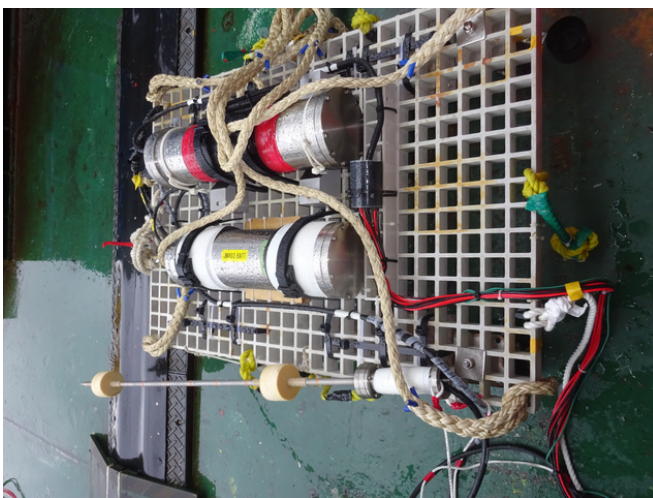
Fig.3.1.9 Photo of a electrometer system with heat-flow meter for the long-term monitoring.
