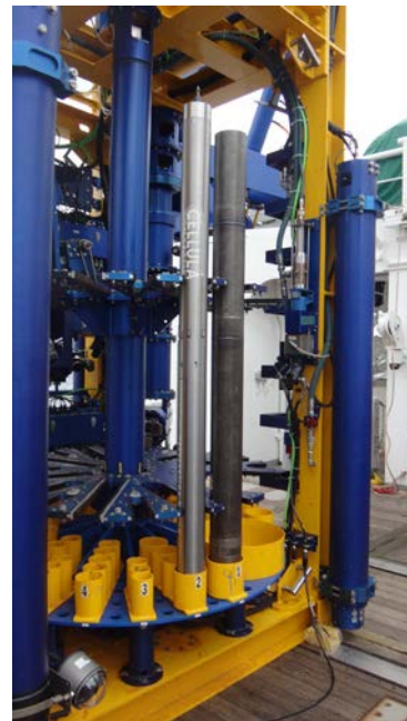
Fig. 3-11 The deployment module was set in the carousel (Silver cylinder)
