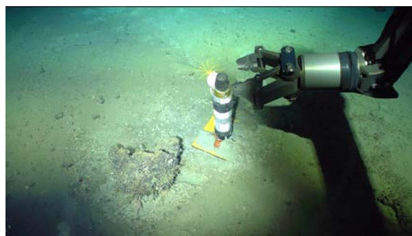
Fig. 3-8 Recovered miniature transponder ID:65
