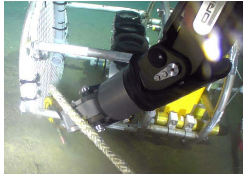
Rope hooking by the manipulator
