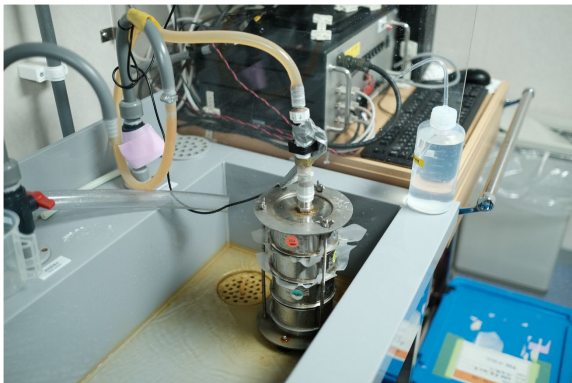
Pumped Seawater-Microplastic sampler
