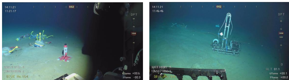
Fig. 7 The Lily tilt-meter site (left) and the equipment for deployment
