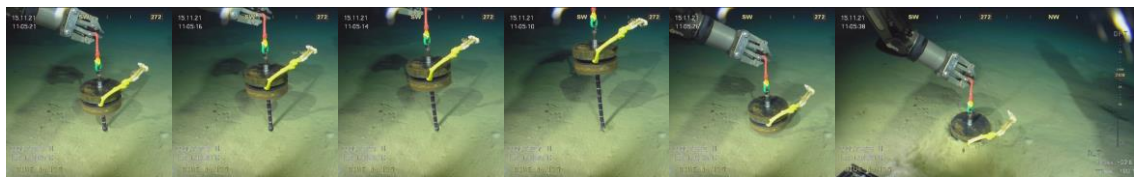
Fig. 9 Stiffness test using dead-weight stick at 2F-S2 site
