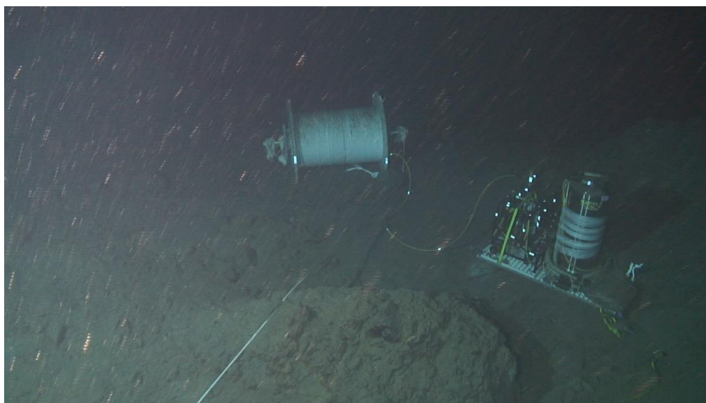
Fig. 2 Observatory equipment (left: cable drum, right: sensor system) of the KMC-10 station
