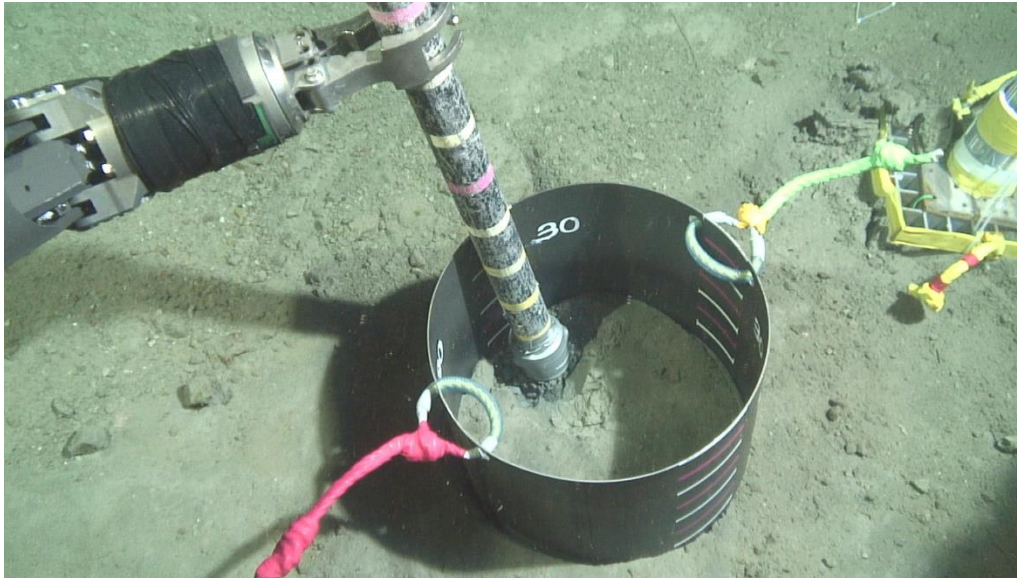
Fig. 3 Casing installation test by the suction system
